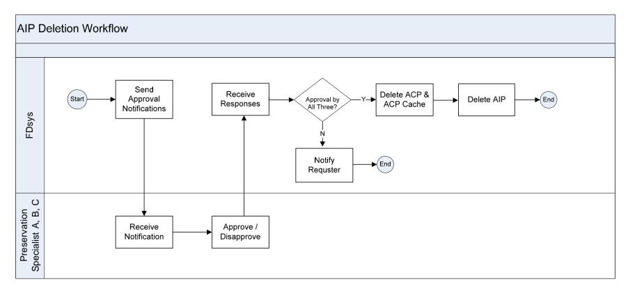
Figure 8.7-1 AIP Deletion Workflow
