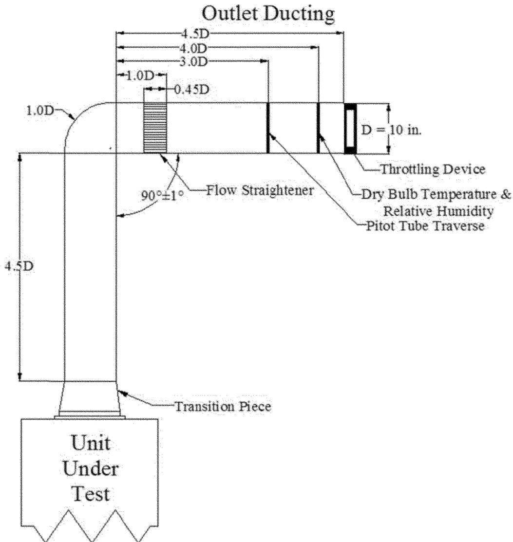
Figure 3: Outlet Vertical Duct Configurations and Instrumentation Placement
