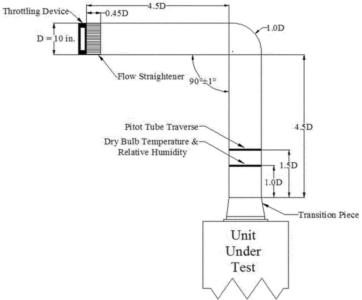
Figure 2: Inlet Vertical Duct Configuration and Instrumentation Placement
