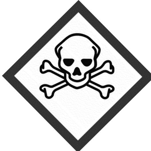
(b) Each side of the marking shown must be at least 100 mm (3.9 inches).
