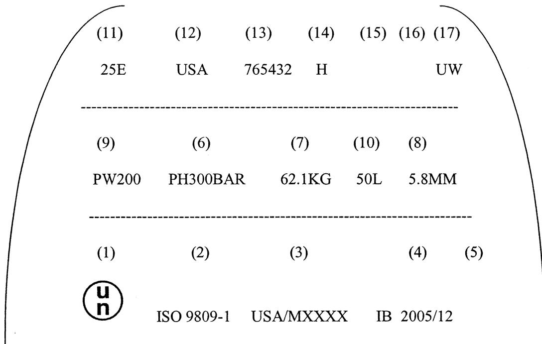
(q) *Other markings.* Other markings are allowed in areas other than the side wall, provided they are made in low stress areas and are not of a size and depth that will create harmful stress concentrations. Such marks must not conflict with required marks.
