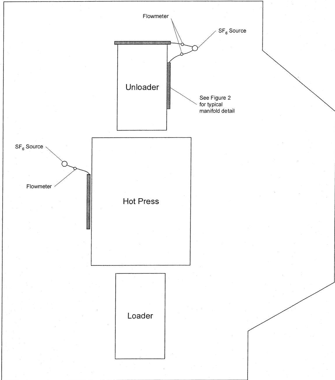
Figure 1. Plan view schematic of hot press and enclosure showing SF<sub>6</sub> manifold locations.
