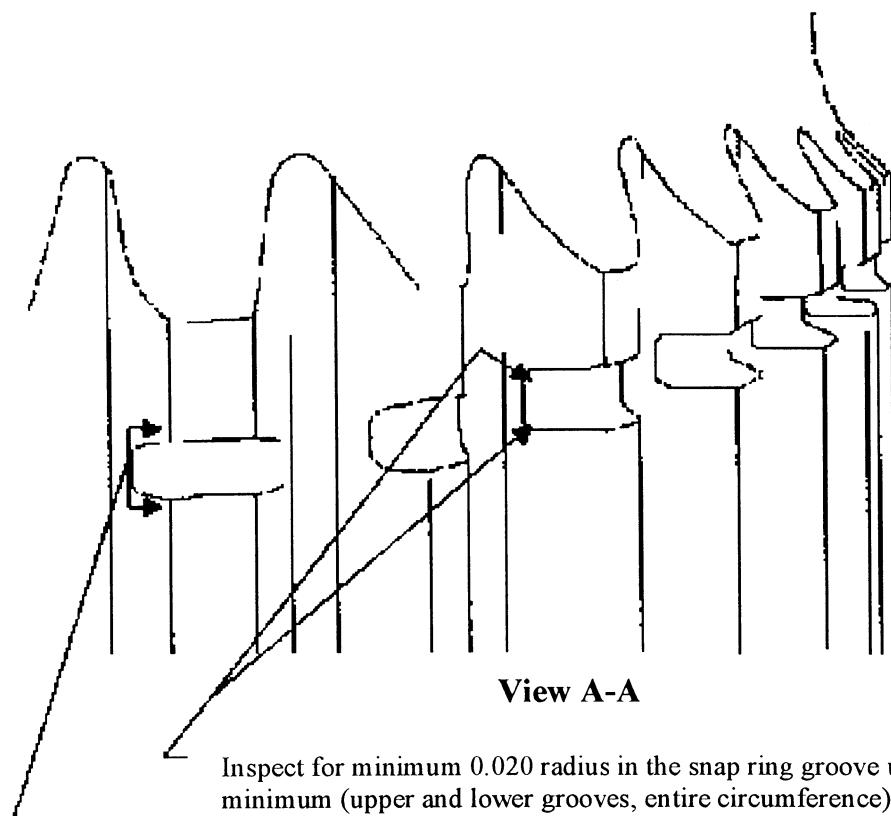
Inspect for minimum 0.020 radius in the snap ring groove using 100x magnification minimum (upper and lower grooves, entire circumference)
