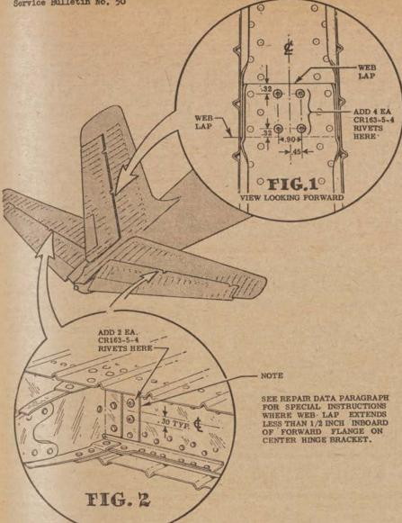
An inspection should be made immediately to determine if any of the above rivets are missing. If any or all of these rivets are missing the following rework should be accomplished as soon as possible but not later than March 31, 1959.
