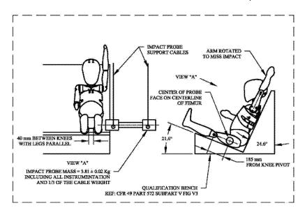
Figure W11. Pelvis lateral impact test set-up specifications.
