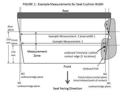
Plan view of a seat showing several example measurement locations for the determination of seating surface width. Measurement 1 is the seat surface width for this illustration.
