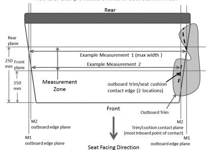
FIGURE 1: Example Measurements for Seat Cushion Width
