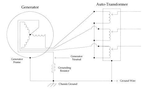
Note that the grounding resistor must be mounted on the same frame with the generator.
