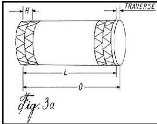
Patent '551 first requires the measurement of the average length of the roll on which the netting sits ( $O$  in Figure 3a) and the length of the entire netting from the two extreme franzes ( $L$  in Figure 3a). The length measurement must then be divided by the number of franzes, minus one, in order to calculate the average length between the franzes ( $H$  in Figure 3c).
