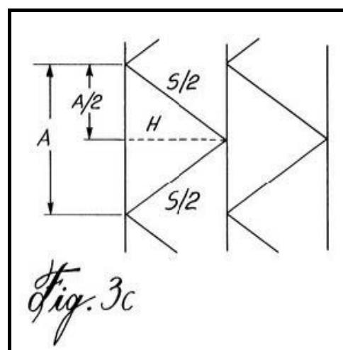
Second, the '551 patent calls for the unrolling of the netting to allow for the measure of ten bases (10A in Figure 3b). A base, in this sense, is the length of the Franz between two Shusses. The total measurement of the ten bases is then divided by ten to calculate an average base (A in Figure 3c).
