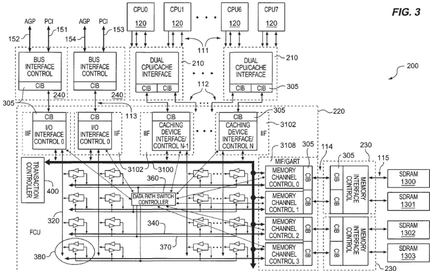
memory devices (1300-1303) exchange data with, and communicate through, processor interfaces (DCIU 210) and memory interfaces (MCU 230). See '442 patent at col. 2, ll. 60-67.
