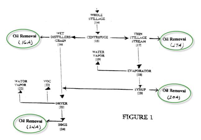
Id. The Oil Removal point labeled "20A" is from the syrup after the evaporator. Id.
