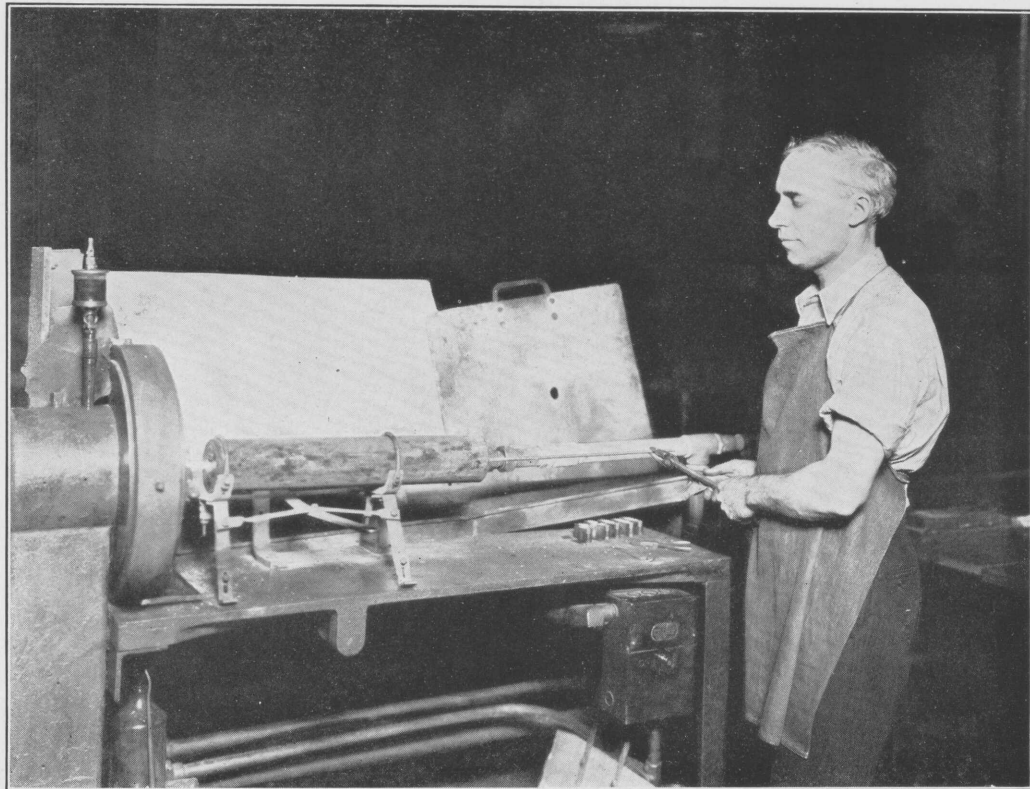
FIGURE 8.—SWAGING TUNGSTEN RODS TO STRENGTHEN METAL FOR MAKING FILAMENTS.
