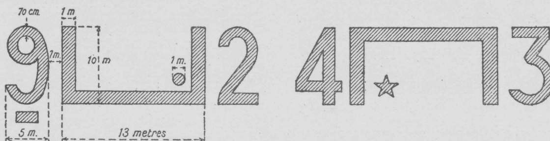
Arrangement of mark for south half of unit sheet. The short sides of the frame shall be oriented true north-south.
