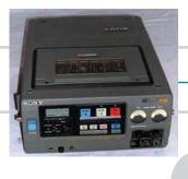
1971 Video Cassette Recorder (VCR): The Sony U-matic VCR, introduced in Tokyo in September 1971, was the world's first commercial videocassette format.
