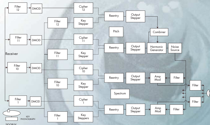
Figure 3: X System receiver (From A History of Engineering and Science in the Bell System, 1925-1975, M.D. Fagen, editor, 1978)
