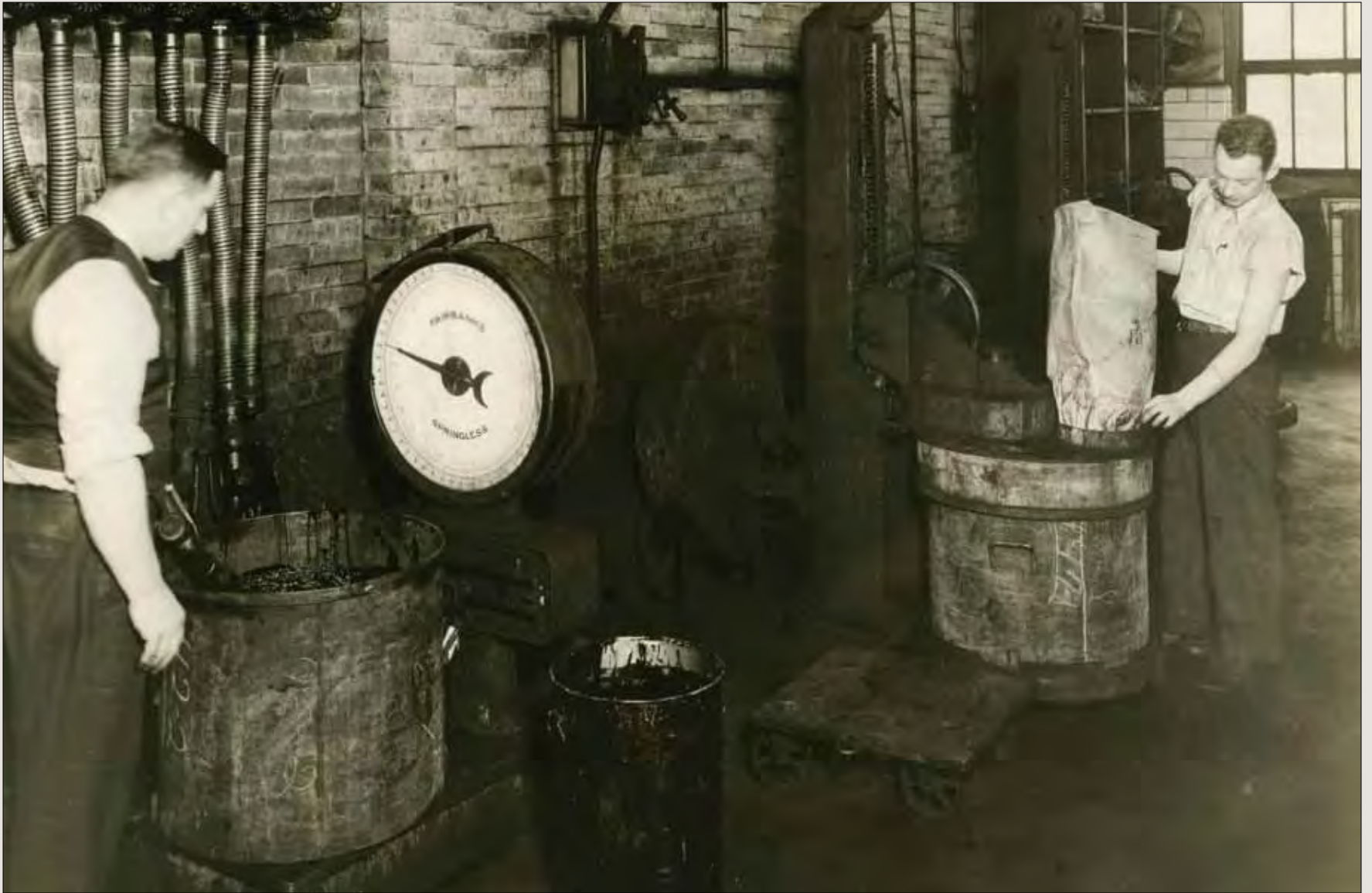
Among its varied responsibilities, the Testing Division was responsible for the manufacture of printing inks. In this photo from the 1930s, pigment is mixed with solvents piped by gravity to the 5th floor from tanks on the 6th. The machine at right is a mixer.
