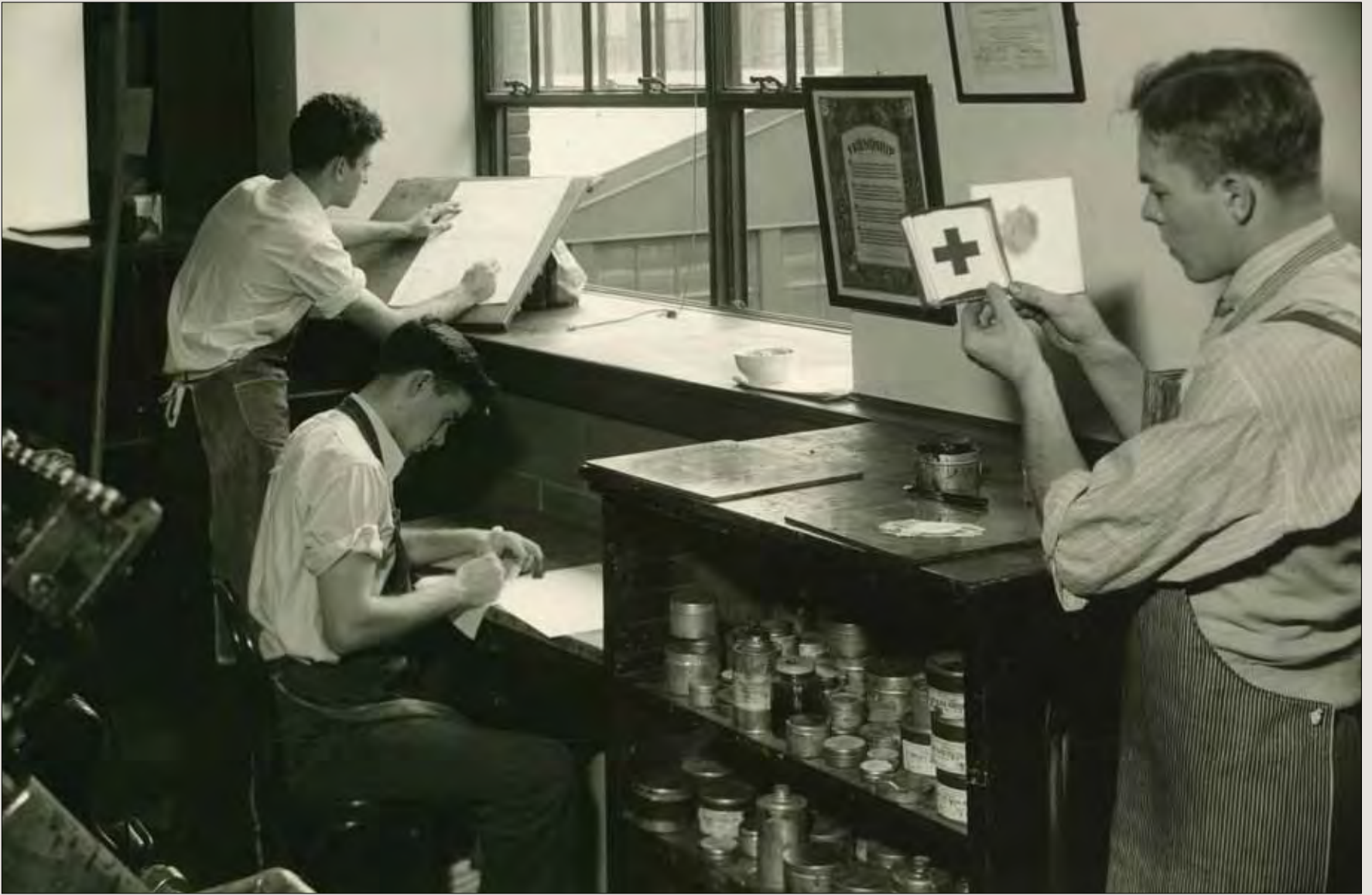
These apprentice pressmen are checking color match and density of printing ink in the apprentice job press room.
