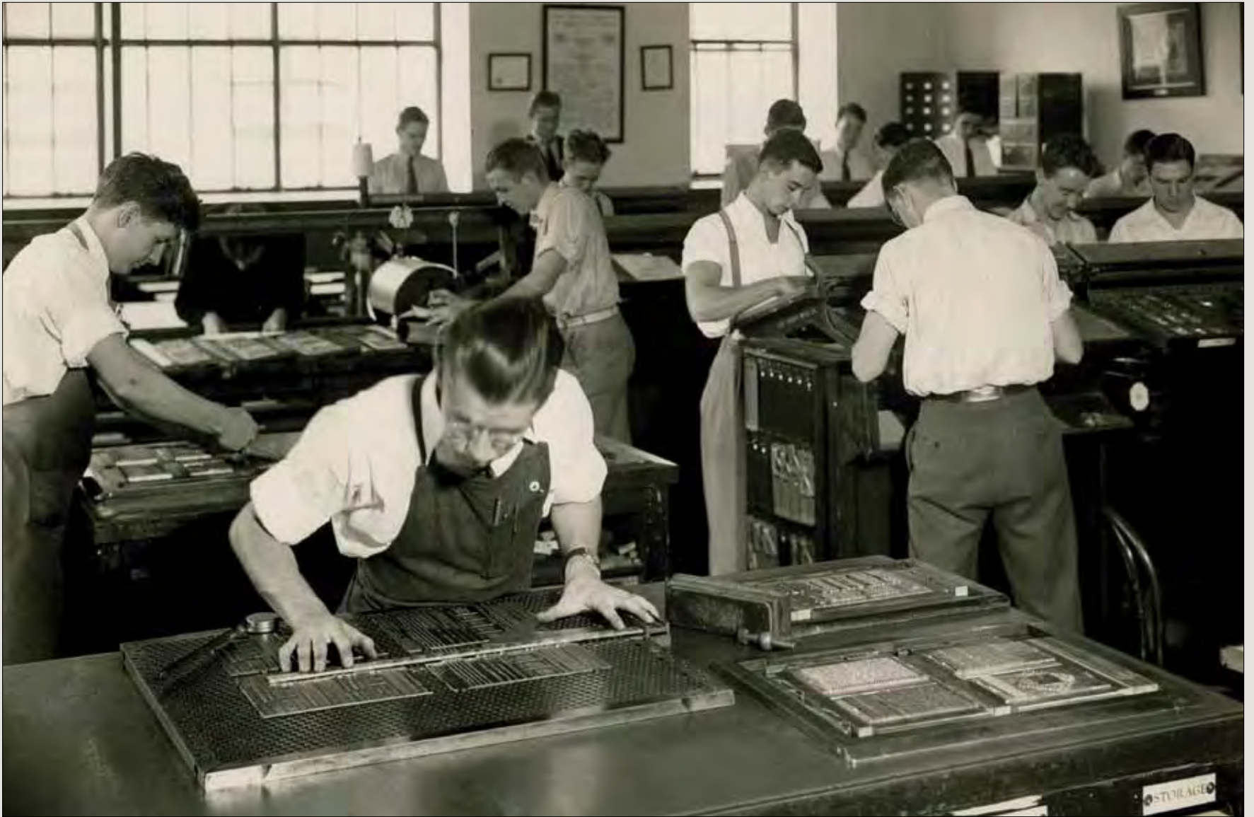
Electrotype plates are imposed into page forms.
