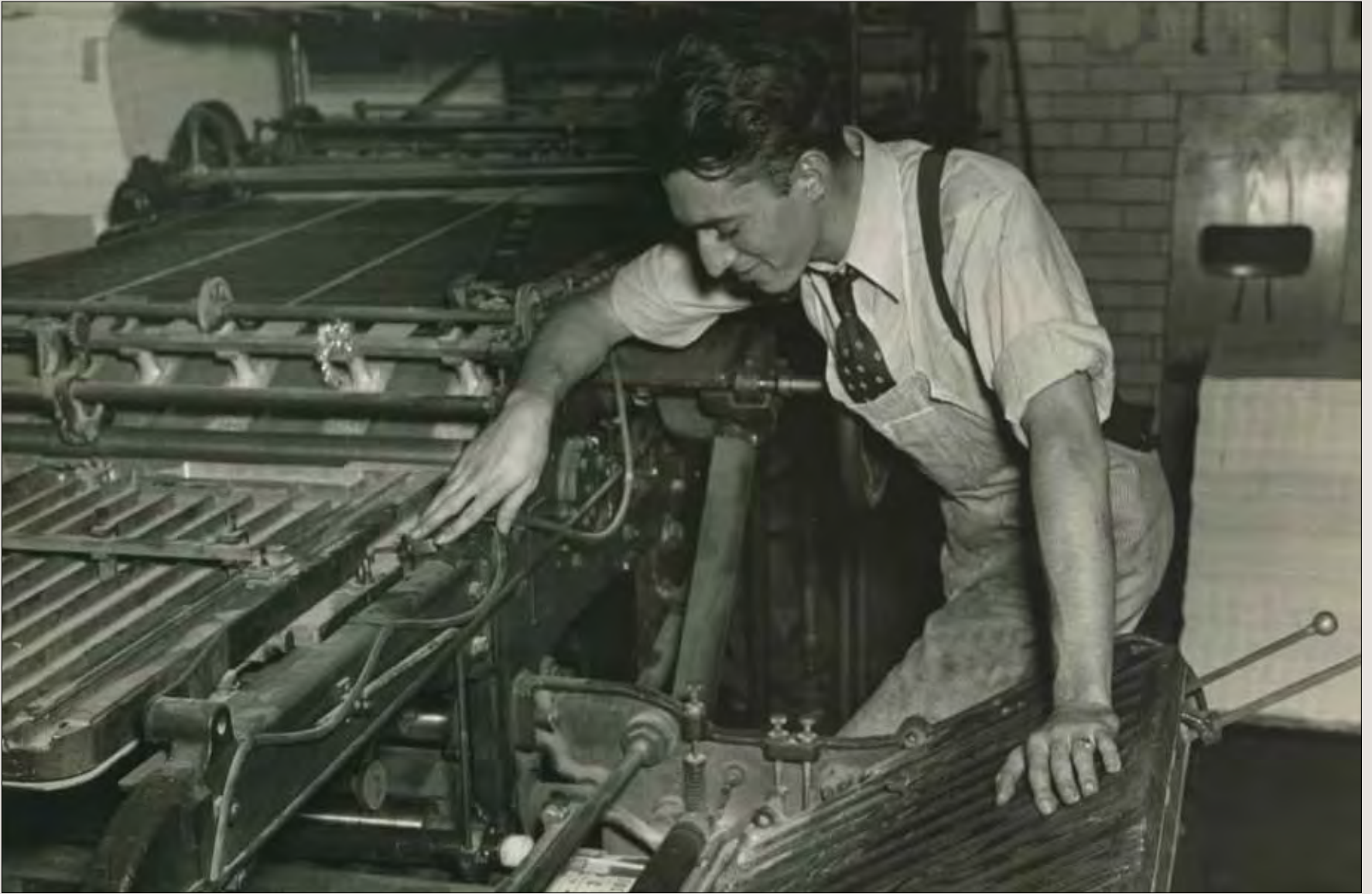
Apprentices were also trained as bookbinders. Here an apprentice operates a Cleveland folding machine.
