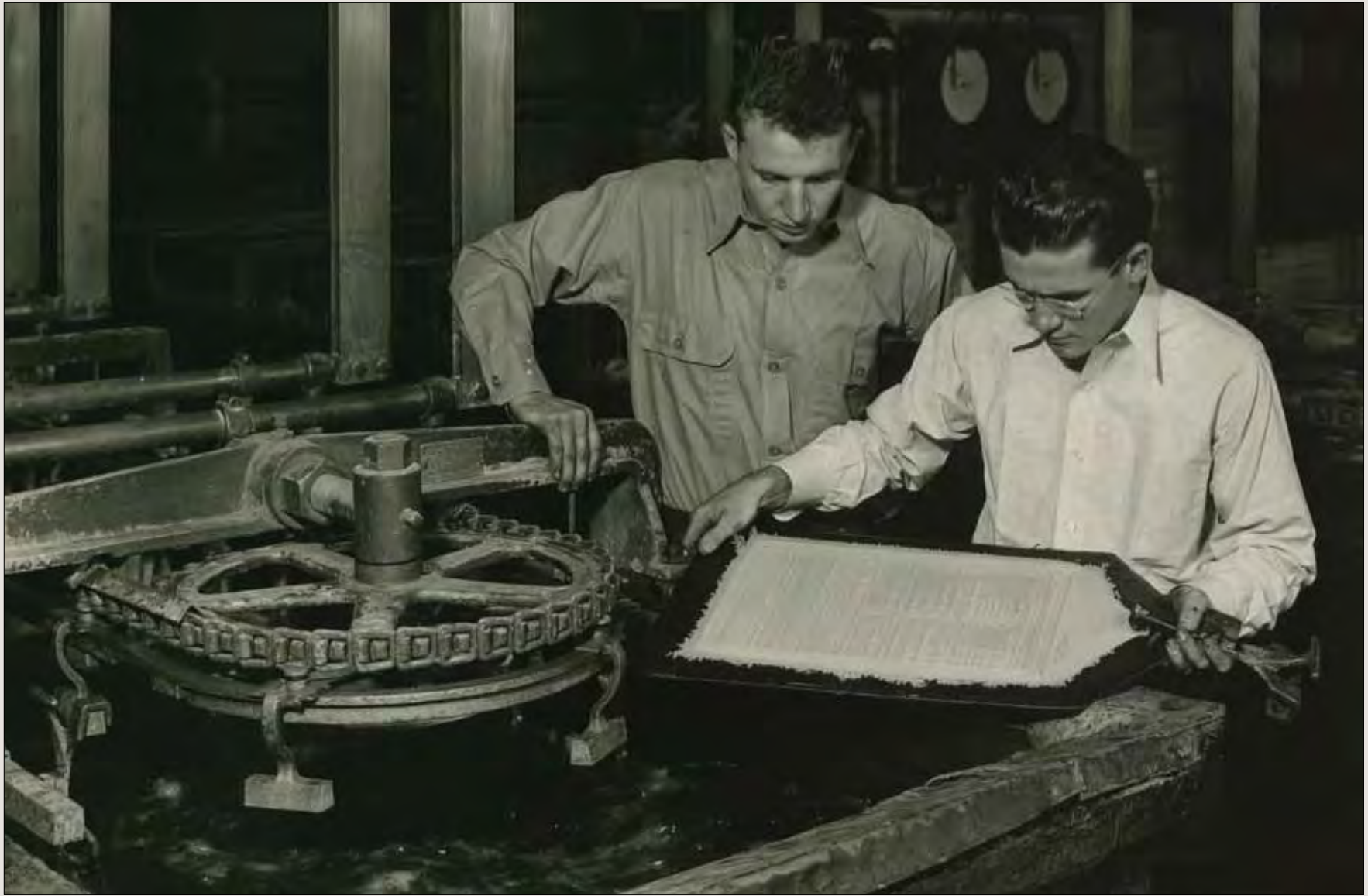
Apprentices inspect a plate which has been immersed in the etching tank.
