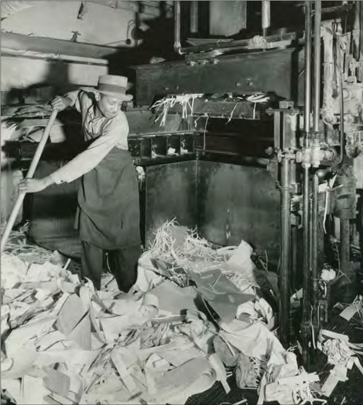
Production of printed documents inevitably generates paper waste. In this photo from the 1940s, waste paper is forked into a baling machine in preparation for being shipped to a mill to be pulped and (in modern terms) recycled.
