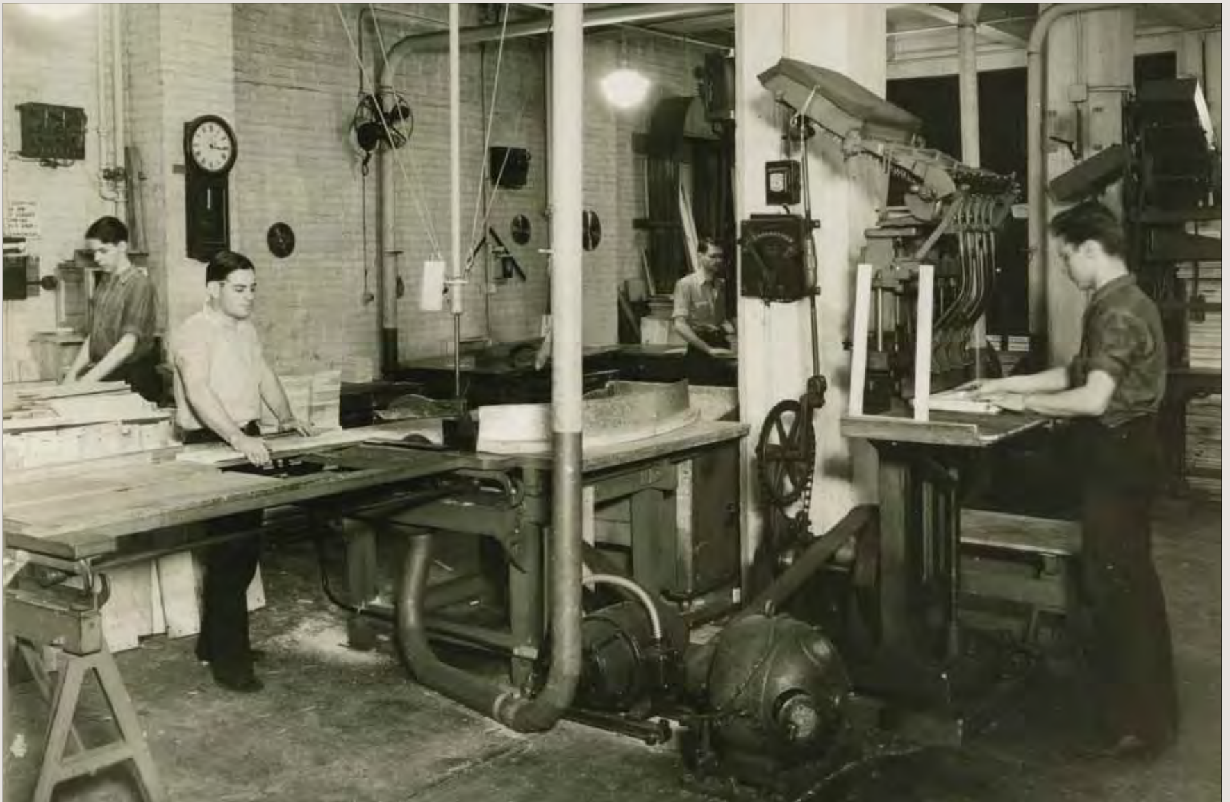
Because of the size and complexity of its operations, and the demanding requirements for quick delivery, GPO developed a culture of “making it here,” which stretched from inks and adhesives to furniture and crates. Here carpenters are using special machines for making shipping boxes. Photo circa 1930.
