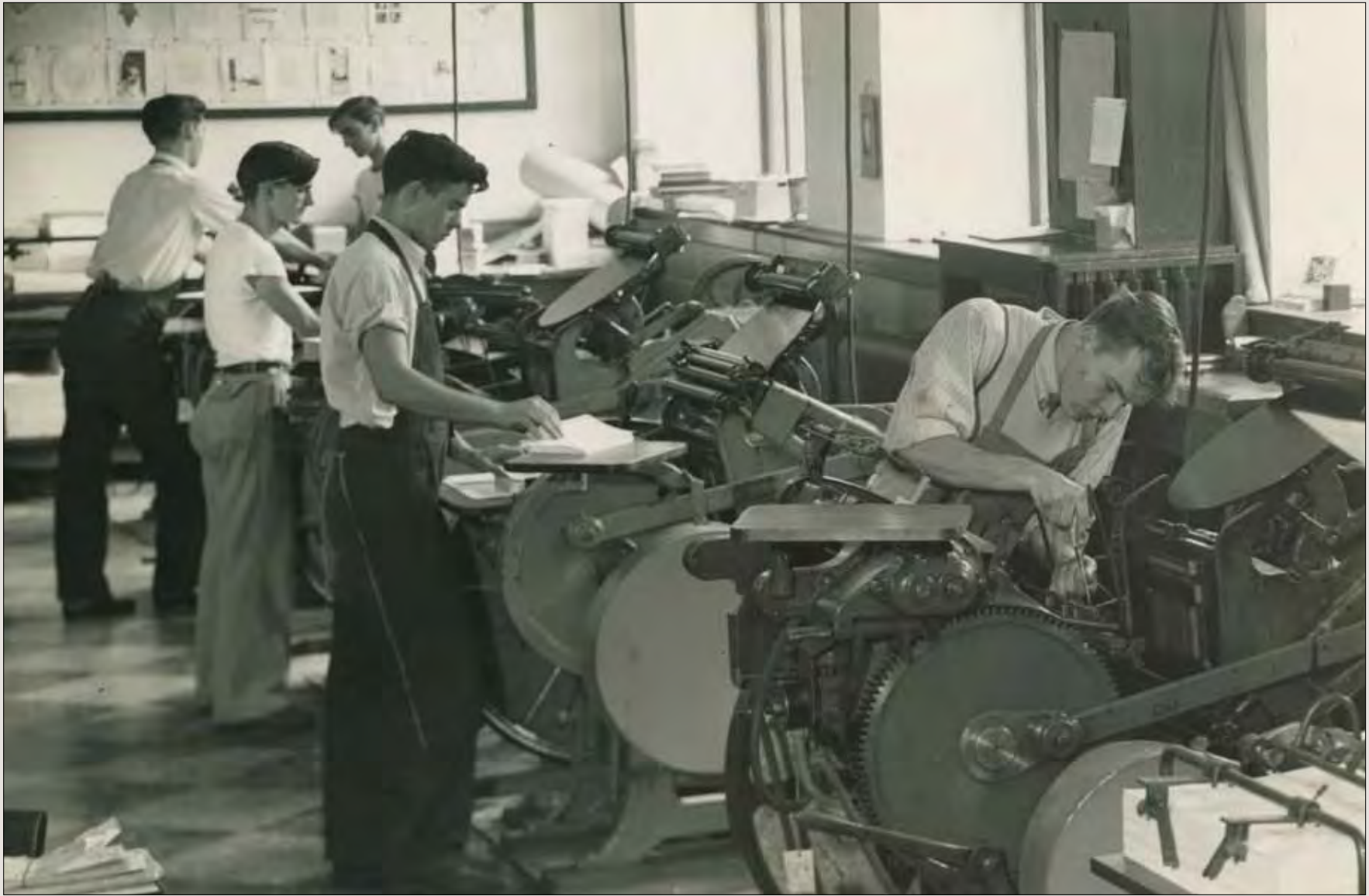
Apprentices eventually were cleared to operate all types of presses, like these platen presses in the job shop.
