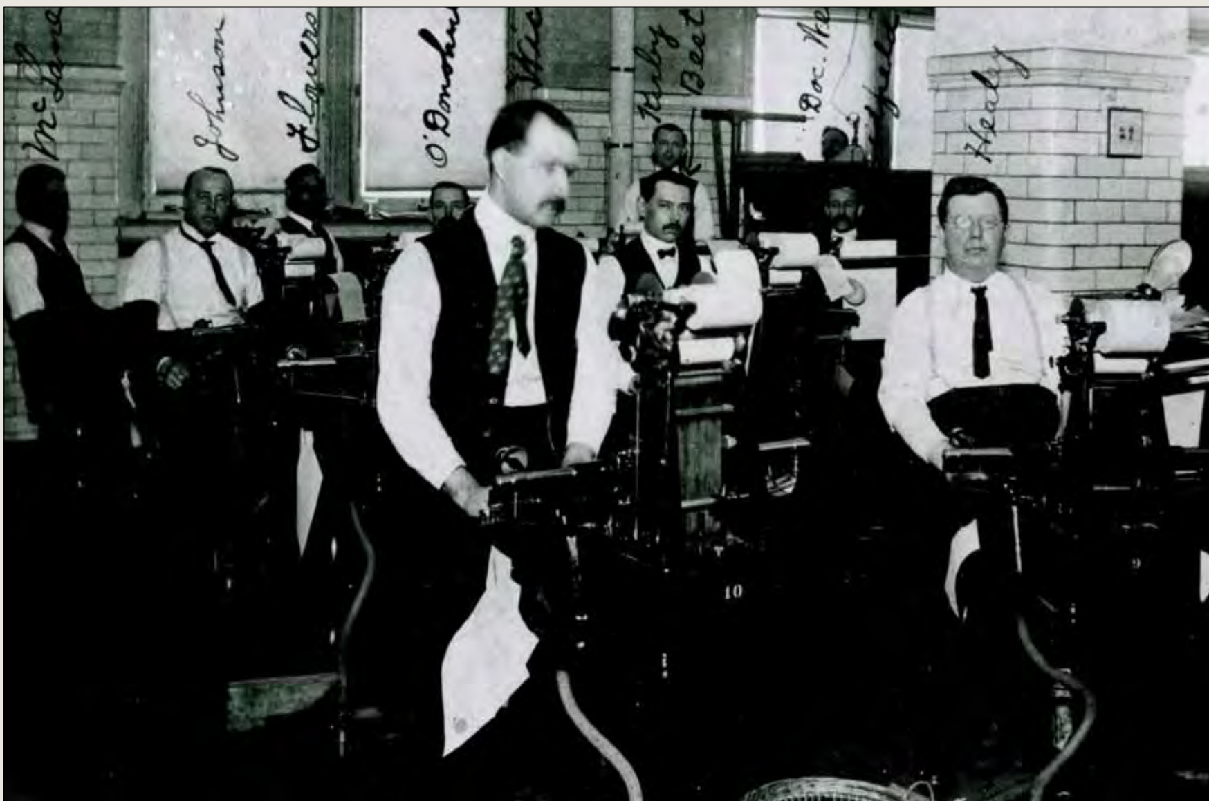
In 1904, the two most successful systems for setting type by machine were introduced to GPO: Monotype and Linotype. Monotype, which cast individual characters in metal, arrived with 28 machines “on trial.” This photo shows 10 of the first Monotype operators, journeymen originally trained as hand compositors.
