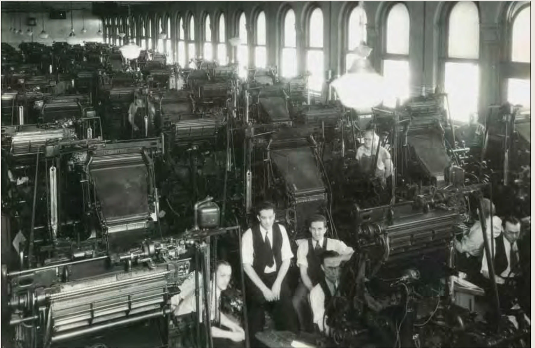
By the 1920s and '30s, when this photo was taken, there were 100 or more Linotypes at GPO. Each machine weighed over 2400 lbs.
