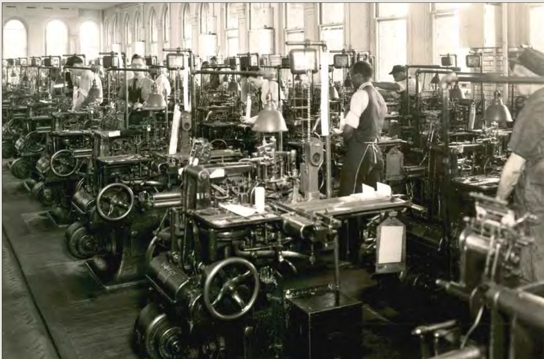
Casters could be set up for composition (producing galleys of sorts, properly spaced) or for sorts (producing letters, punctuation, etc.) that could be inserted by hand to correct mistakes in galleys). Photo circa 1930.
