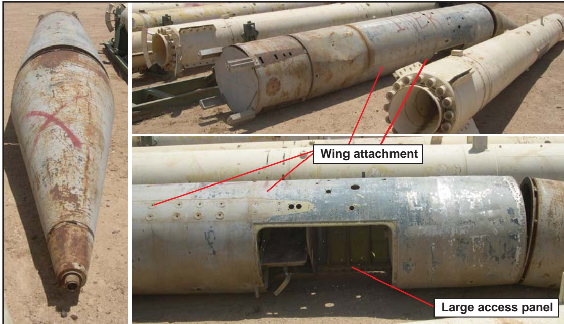
Figure 3. Early Al Samud II using HY-2 airframes.
