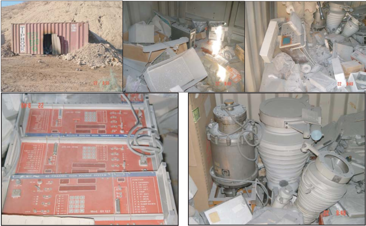
Building 163 (connex): Shipping crate (connex) (top left), digital equipment (top center and top right), high-voltage system (bottom left), and vacuum pumps (bottom right).
