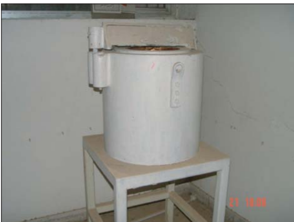
Building 59: Rad. source-led cave (R45).
