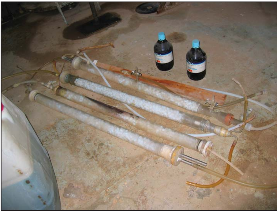
Figure 25. Packed columns used in phosphoric acid purification studies conducted at Ibn Sina in the mid-1990s (photo taken by ISG Team, December, 2003).
