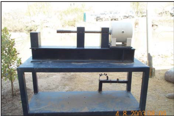
Figure 31. Technical Research Branch facility inspection—shock impact materials test rig.
