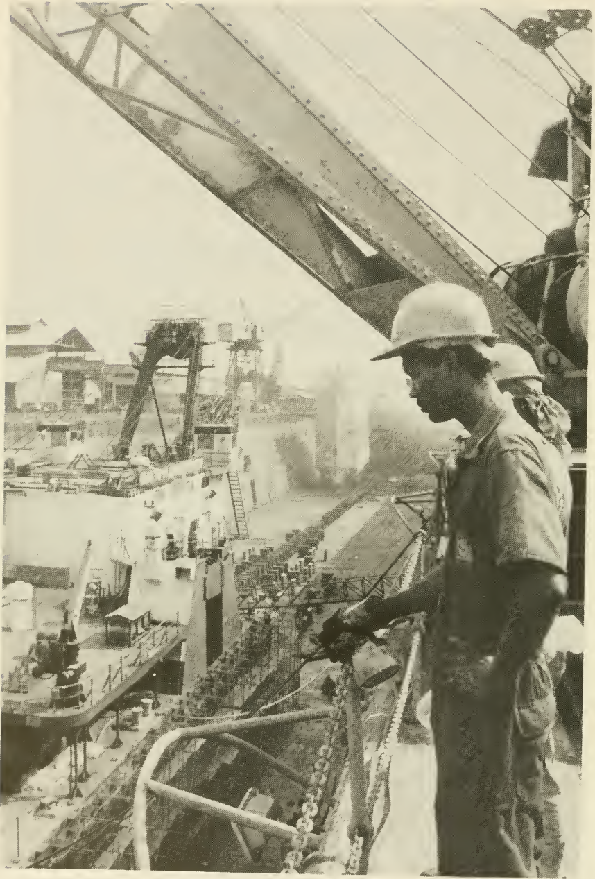
Contract workers look on as the Commission's dipper dredge RIALTO M. CHRISTENSEN (foreground) and Floating Caisson #2 (background) undergo one phase of a major overhaul at the Balboa drydock. The other phase of the overhaul work was performed at the Industrial Division at Mt. Hope.
