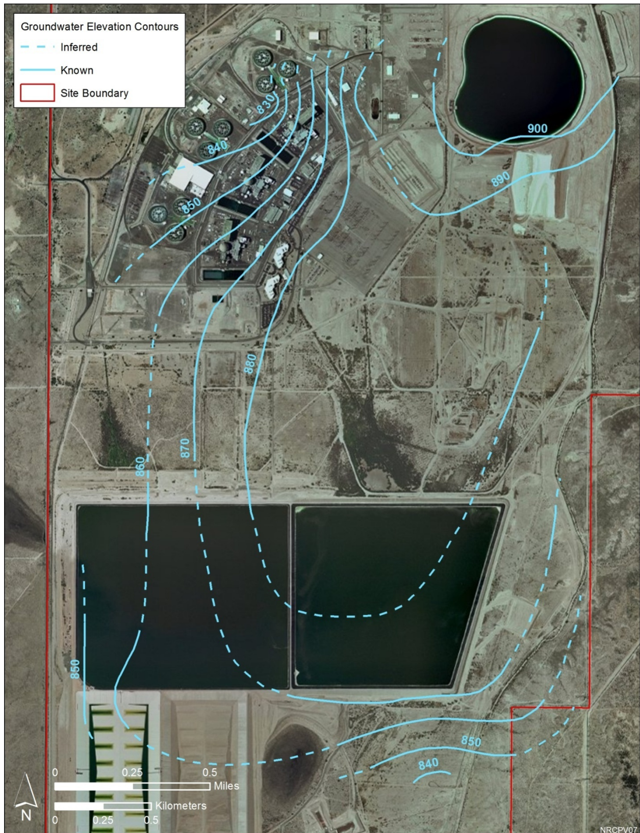
Figure 2.2.3-2 Groundwater Flow in shallow aquifer below PVNGS (APS 2009c)
