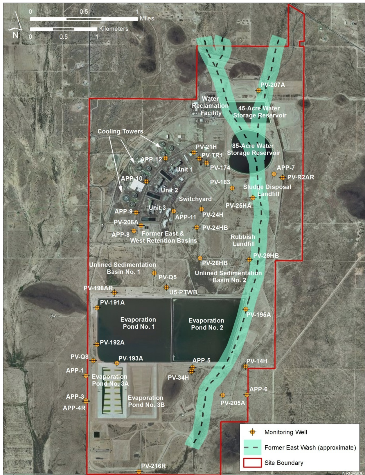
Figure 2.1.7-1 PVNGS Surface Impoundments, Landfills, and Monitoring Wells
