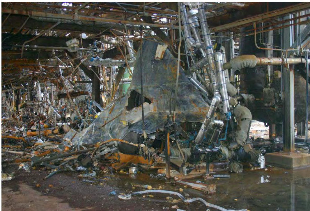
Figure 1. Residue treater came to rest inside the Methomyl-Larvin unit
