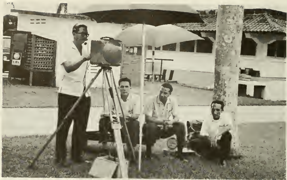
The instrument is a tellurometer and using it is Julio Mock, a student from Panama in the Field Surveys Branch of the IAGS school. Seated, from left: Jose Whittingham, assistant instructor, also from Panama; Nelson Rada of Venezuela; and Victor Villatoro of Guatemala.
