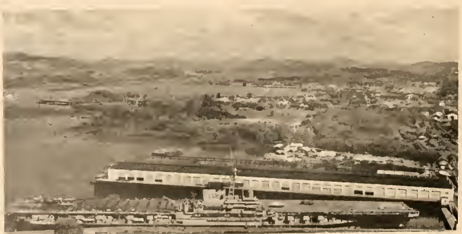
BIGGEST SHIP ever to dock in Balboa is the U. S. Aircraft Carrier Franklin D. Roosevelt , shown here alongside the docks. The 45,000-ton ship is 968 feet long and has a 113-foot beam—too wide to pass through the Canal locks. The carrier made her intercoastal trip via Cape Horn.
