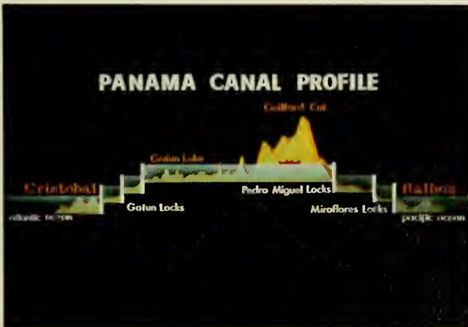
Ships transiting the Canal are raised and lowered 85 feet, from sea level to sea level, by a system of three sets of locks.
