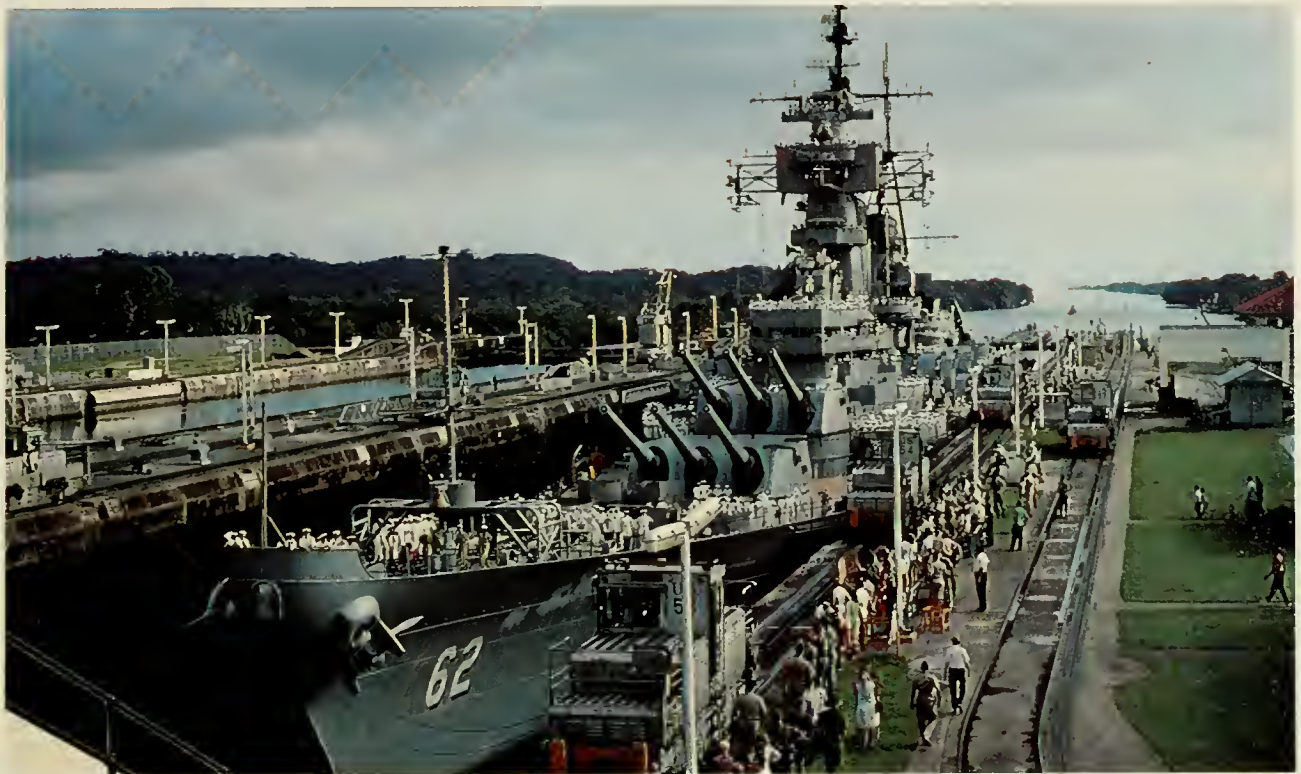
Filling the east chamber at Pedro Miguel Locks with her 108-foot beam is the battleship "New Jersey", which along with her sister ship, the "Missouri", is among the widest vessels to transit the Canal.
