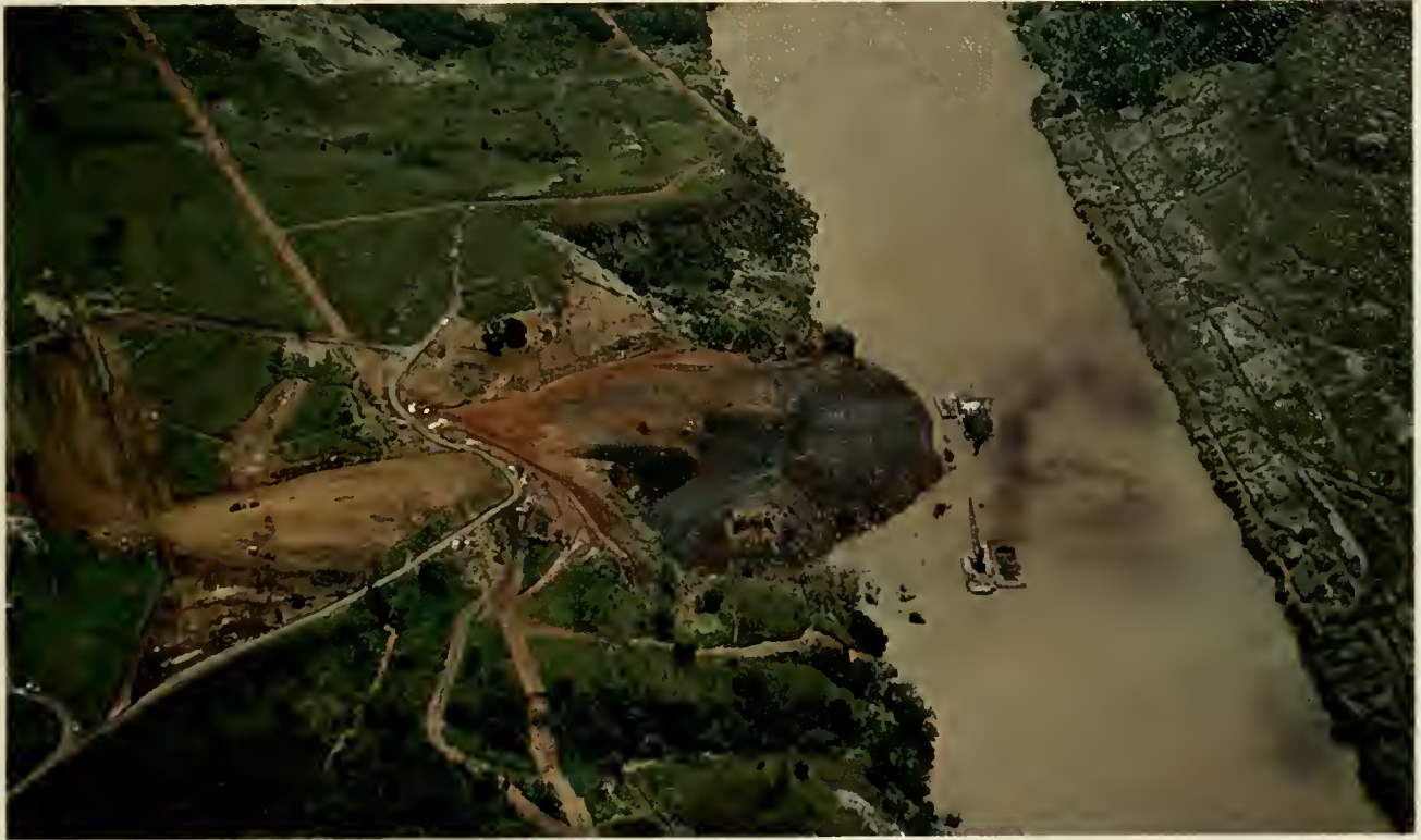
An aerial view of the October 10th slide shows the craneboat "Goliath" and the dipper dredge "Cascadas" starting clearance work.
