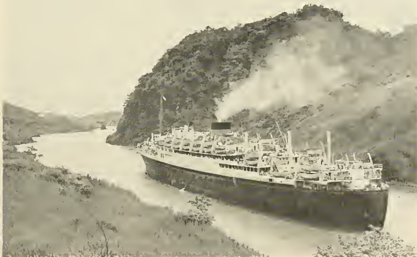
TWO PILOTS are required for ships the size of the 712-foot Georgic , shown here in Gaillard Cut. One pilot alone would not have sufficient visibility to handle a ship of this size and would exhaust himself racing from side to side of its bridge. The Georgic is 27,468 gross tons and has a beam of 82 feet.
