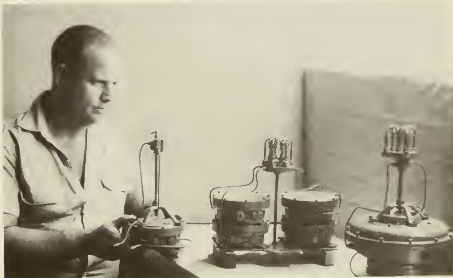
Roy R. Shuey, leader machinist, with, left to right, a fixed single burner light, a double flasher unit with multiple burners, and a single flasher unit for offshore installations having two different characteristics in one lantern. The flasher with multiple burners provides a brighter light than does a single burner flasher.
