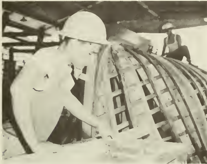
That upside-down boat in the background is the U.S. Tarpon, a mail and freight launch in the making. The young workman in the foreground is Napoleón Myta, a 26-year-old Panamanian who is cutting the framing which will be bent lengthwise over the molds and ribbands of the new launch. He has been with the Canal 6 months and is using skills he learned as a boat builder in Panama as well as new ones he is learning at the Launch Repair Shop.
