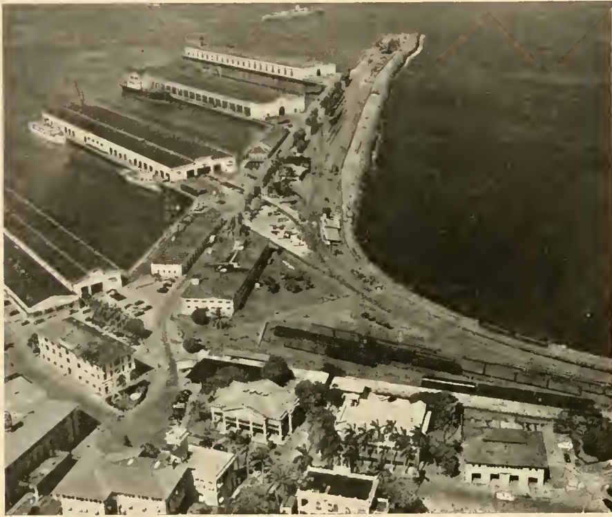
CRISTOBAL PIERS jut out from the mole. They provide more than a mile of berthing space and about 15 acres of covered pier space. Approximately 2,000 of the Canal's employees depend directly on port operations for their livelihood.
