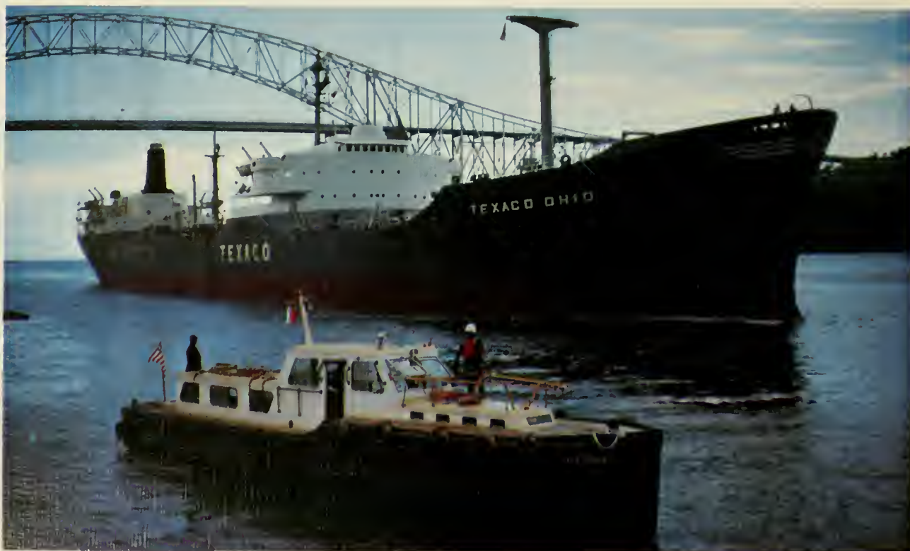
The long, narrow hull of the pilot's launch is built to withstand the rough waters of the outer anchorages.
