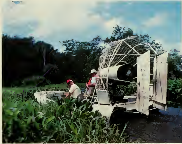
The airboat "Santa Sierra" glides into weed-infested waters to spray herbicide on the floating vegetation that if left untreated would overrun the Canal.
