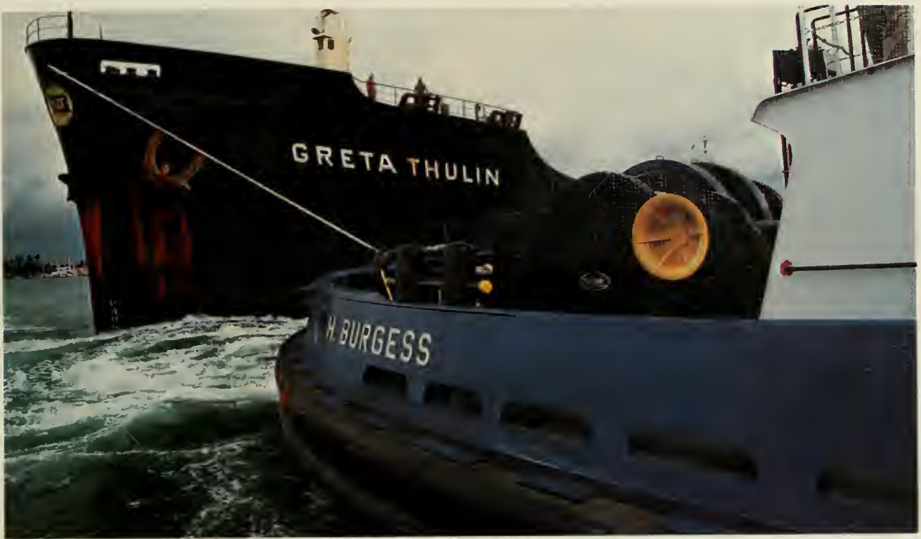
The "H. Burgess" and its sister the "M. V. Walker" are the Canal's first omnidirectional tugs, capable of thrusting their power in any horizontal direction. The tugs are named after the fourth and fifth governors of the Canal Zone.
