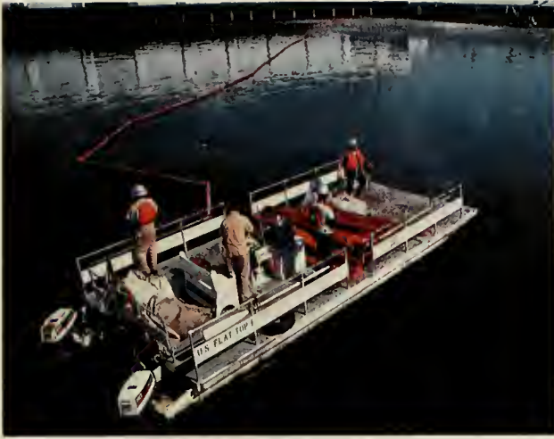
Oil containment boom is deployed from a motorized fiberglass catamaran after a major oil spill in Balboa piers.
