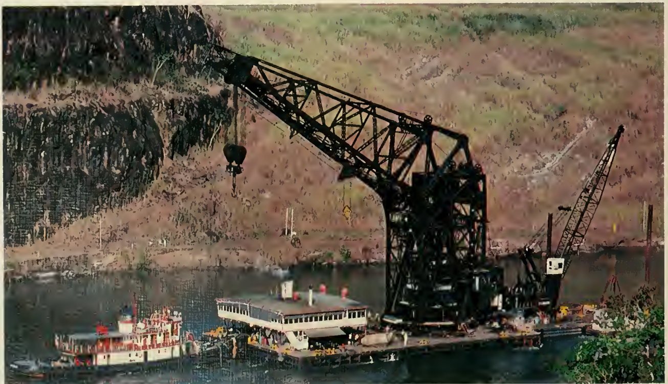
Two Canal giants in a tandem tow, the floating cranes "Hercules," left, and "Goliath" are pushed to a worksite in Caillard Cut by the tug "San Pablo."
