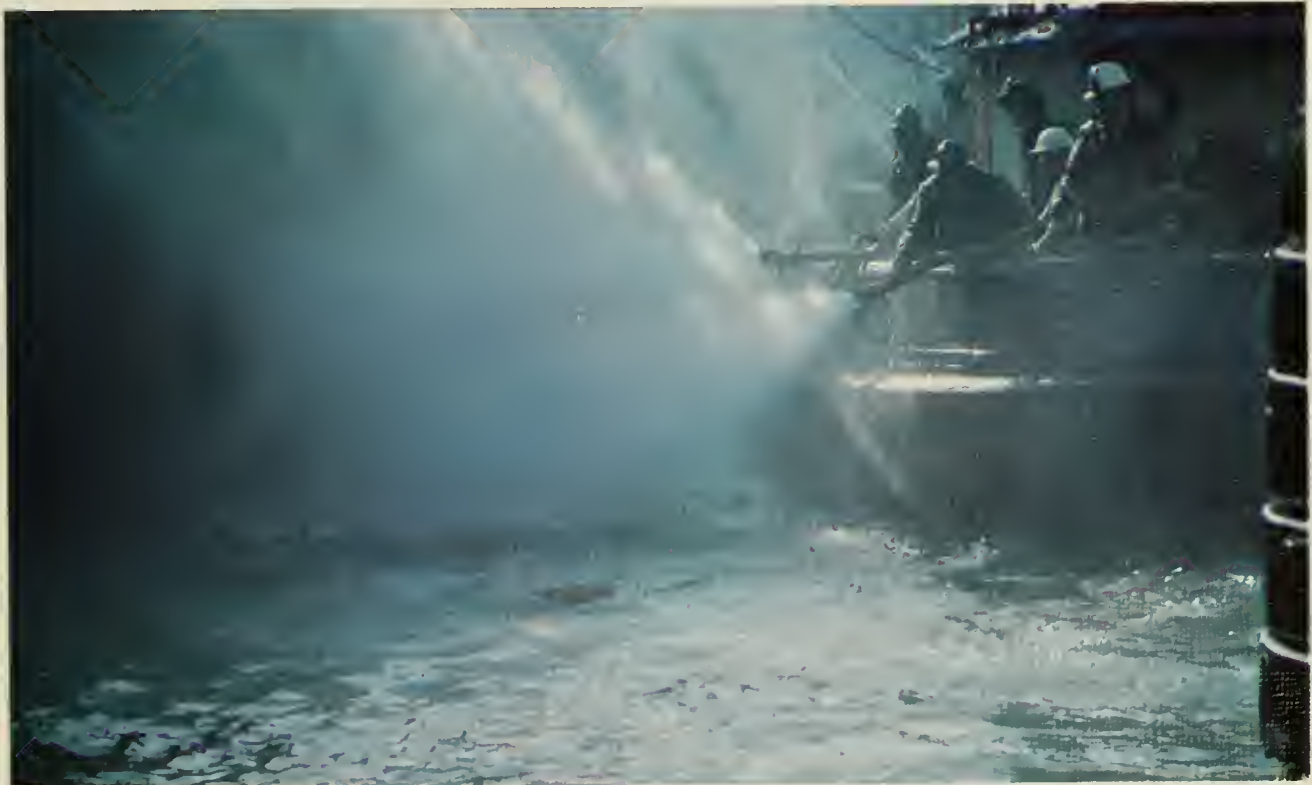
All of the Canal's tugs are equipped for firefighting, having the ability to generate foam from large capacity tanks as well as carrying dry chemicals and being able to pump water directly from the Canal.
