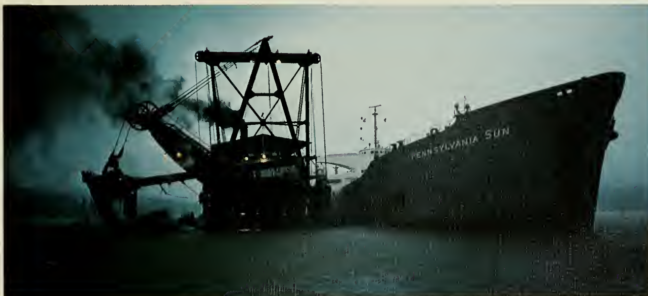
In addition to her duties in construction dredging, the venerable "Cascadas" responds to emergencies. Here the dipper dredge works to free a fully laden oil tanker that ran aground in the Canal.
