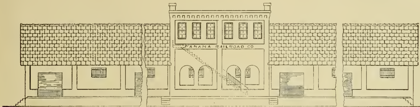
SKETCH A.—FRONT ELEVATION (SECTIONAL) OF NEW PANAMA RAILROAD FREIGHT HOUSE.
