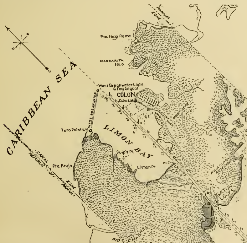
MAP SHOWING AREA OF CONSTRUCTION OF SHORE DIKES IN LIMON BAY. (Dikes are directly west of range light No. 2, and groins are built as far as Limon Point.)
