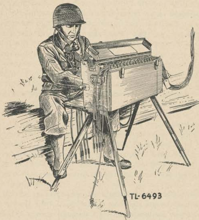
Figure 7.—Switchboard BD-72 set up for operation, showing terminal compartment open.
