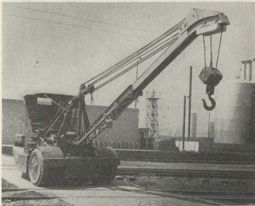
FIGURE 30.—Tractor crane, 10-ton capacity, showing weighted hook block to facilitate overhauling, and winch tread (independently operated) for miscellaneous applications.
