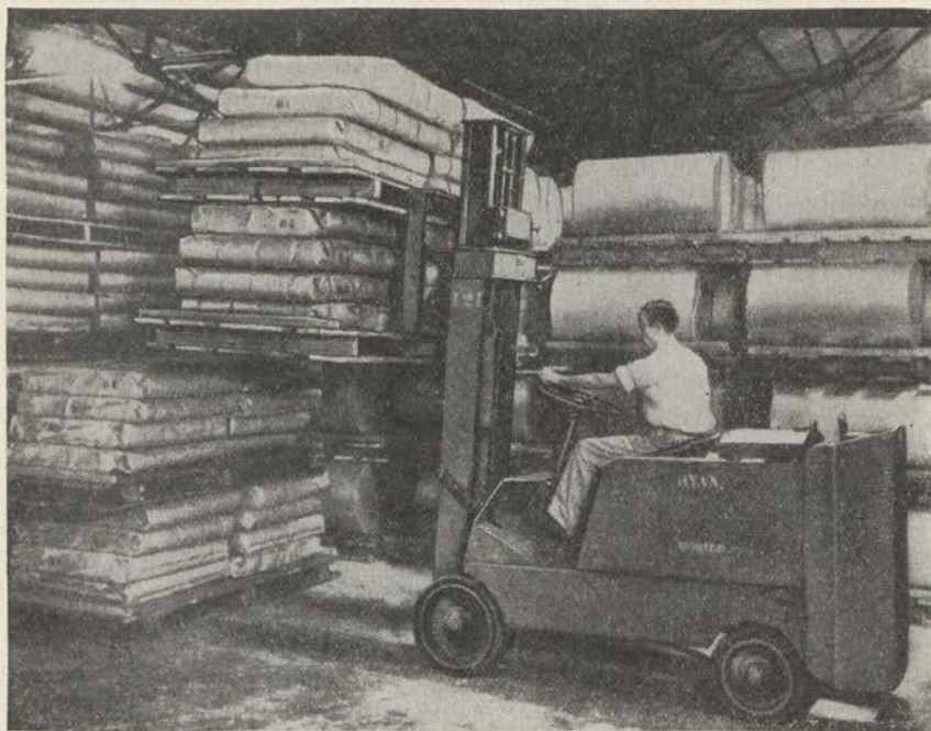
FIGURE 36.—Tiering heavy load.
