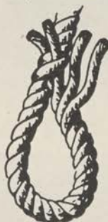
Eye Splice, 4-Stranded Rope.
