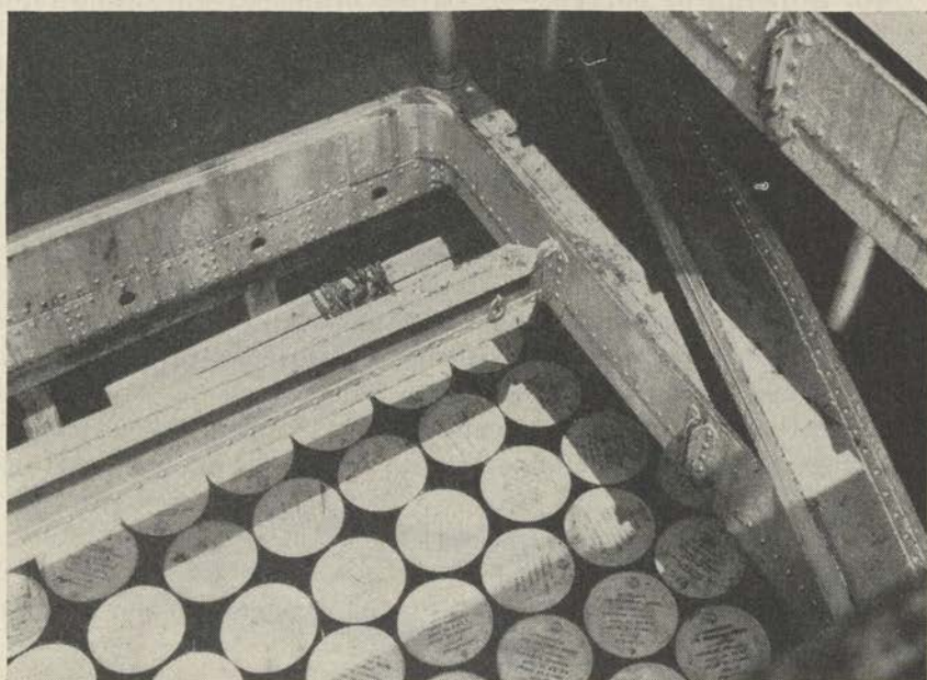
FIGURE 79.—Oil barrels—looking down into partially filled hold. Note one strongback in position, and another lying flat on the 'tween-deck.
