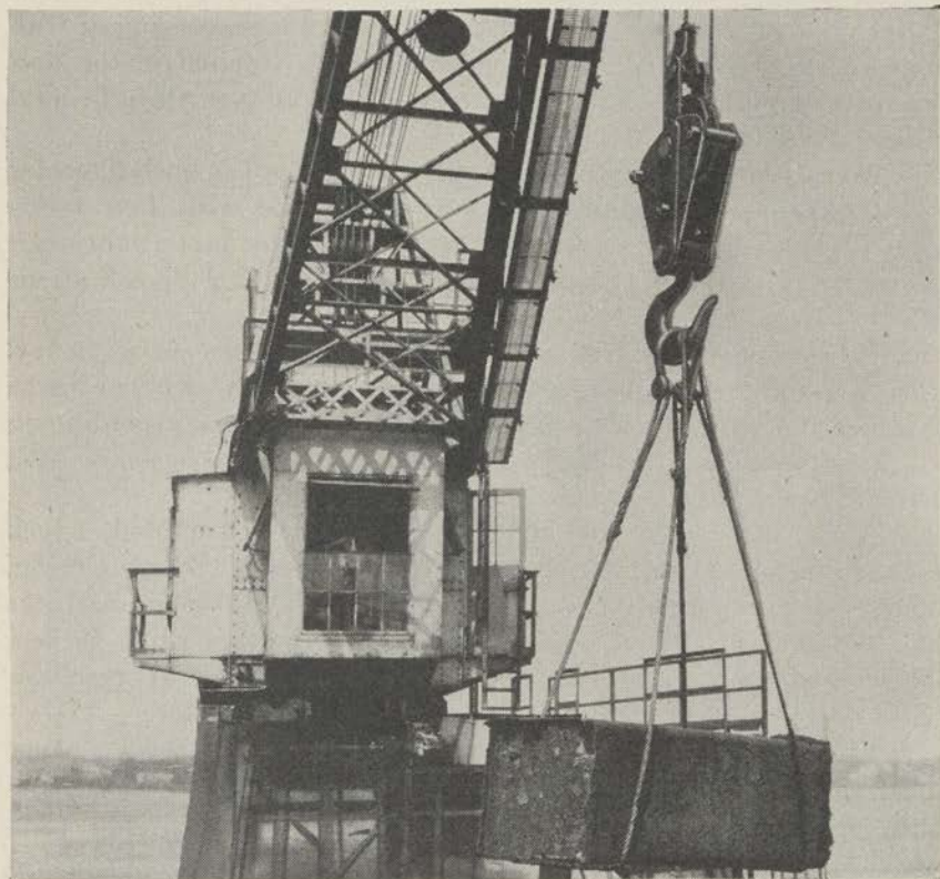
FIGURE 58.—Crane hoist lifting a 3-ton ingot with wire sling.
