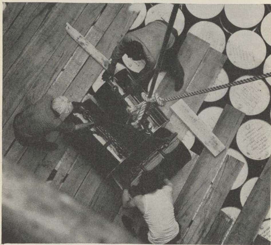
FIGURE 77.—Barrels being lowered into hold. Note planking dunnage on stowed barrels.
