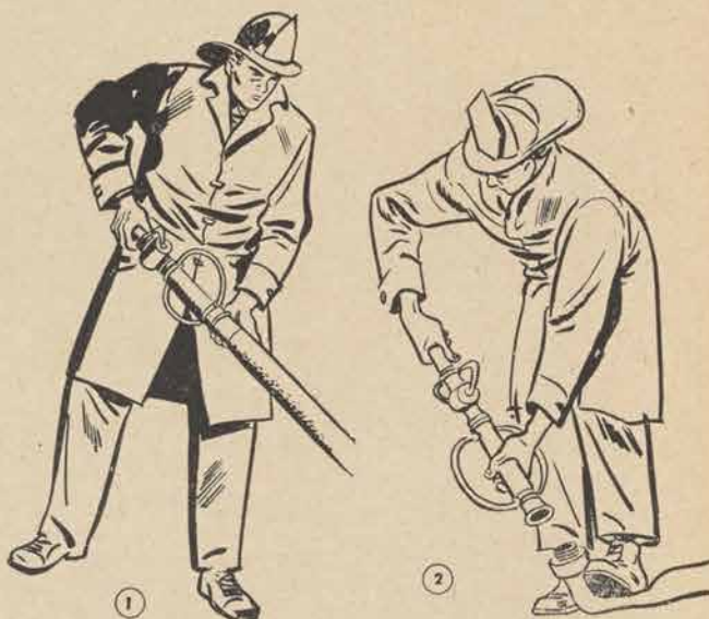
① Left hand is placed on thigh. Nozzle rests on thigh to permit easy alignment for starting threads. ② Holding male end with feet to facilitate attachment. Figure 51. Attaching nozzle. Nozzle must be in shut-off position when not in operation.
