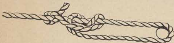
Figure 28. Chimney hitch used to secure rope on which constant strain is placed. Rope can be shortened or lengthened by slipping knot.
