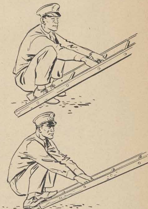
Figure 37. Two methods of footing ladder for two-man raise.
