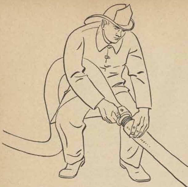
Figure 50. Coupling hose. Male end of hose is in left hand. Hose is supported on hip with right elbow to relieve strain at couplings and free both hands to align and tighten threads.
