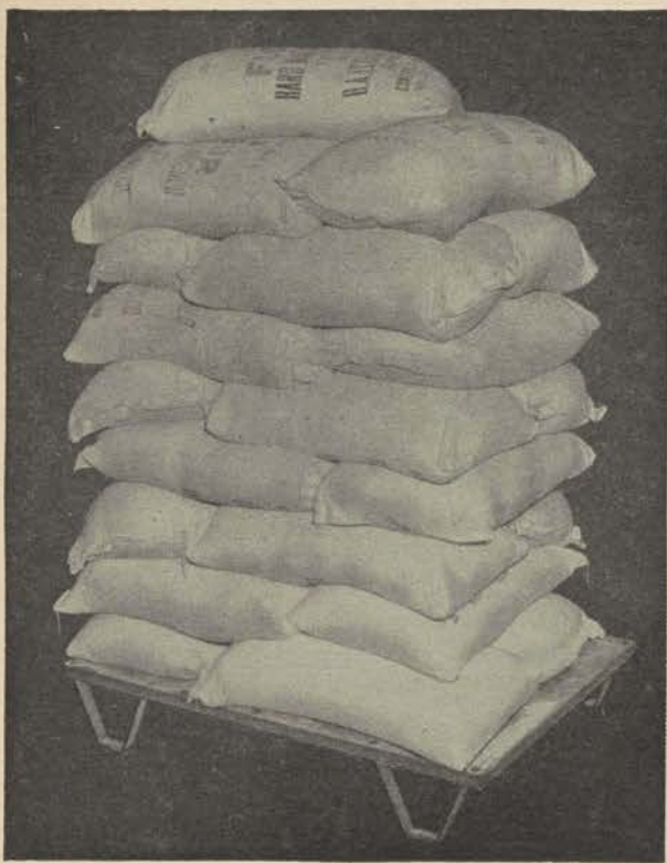
Figure 2. Proper method of stacking flour. The header-and-stretcher method makes a stable stack.
