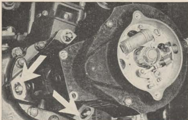
Figure 53. Slotted magneto-housing flange — ignition timing.
