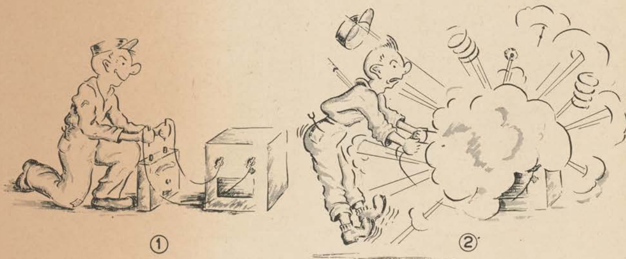
Figure 42. Never connect an ammeter directly across a battery.
