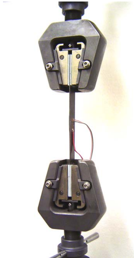
FIGURE 8. TEST SETUP USED FOR THE IN-PLANE SHEAR TESTS
