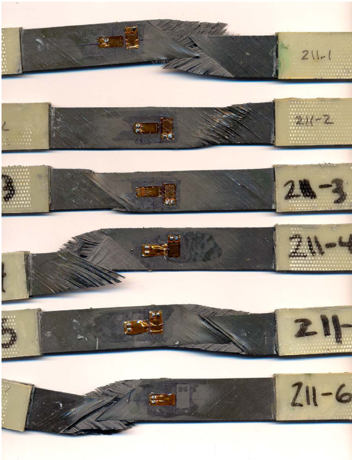
FIGURE A-30. IN-PLANE SHEAR SPECIMENS FROM 16-PLY TAPE LAMINATE TESTED AT 82°C/WET CONDITIONS
