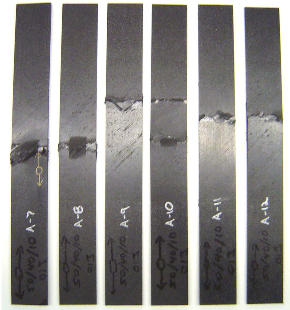
FIGURE A-14. LAMINATE COMPRESSION SPECIMENS FROM 50/40/10 TAPE LAMINATE TESTED ACCORDING TO ASTM D 6484 (SHEAR-LOADED) AT ROOM TEMPERATURE/AMBIENT CONDITIONS
