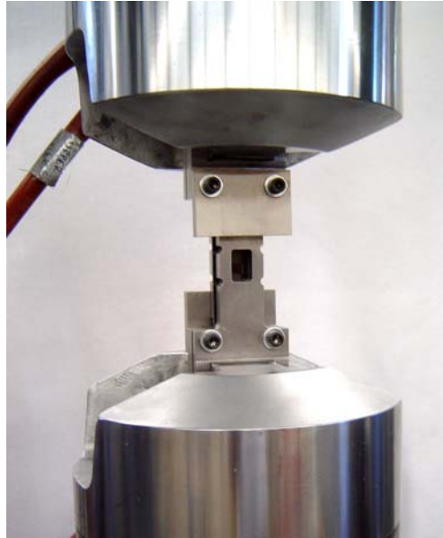
FIGURE 4. SHEAR LOADING OF LAMINATE COMPRESSION TEST FIXTURE USING HYDRAULIC GRIPS
