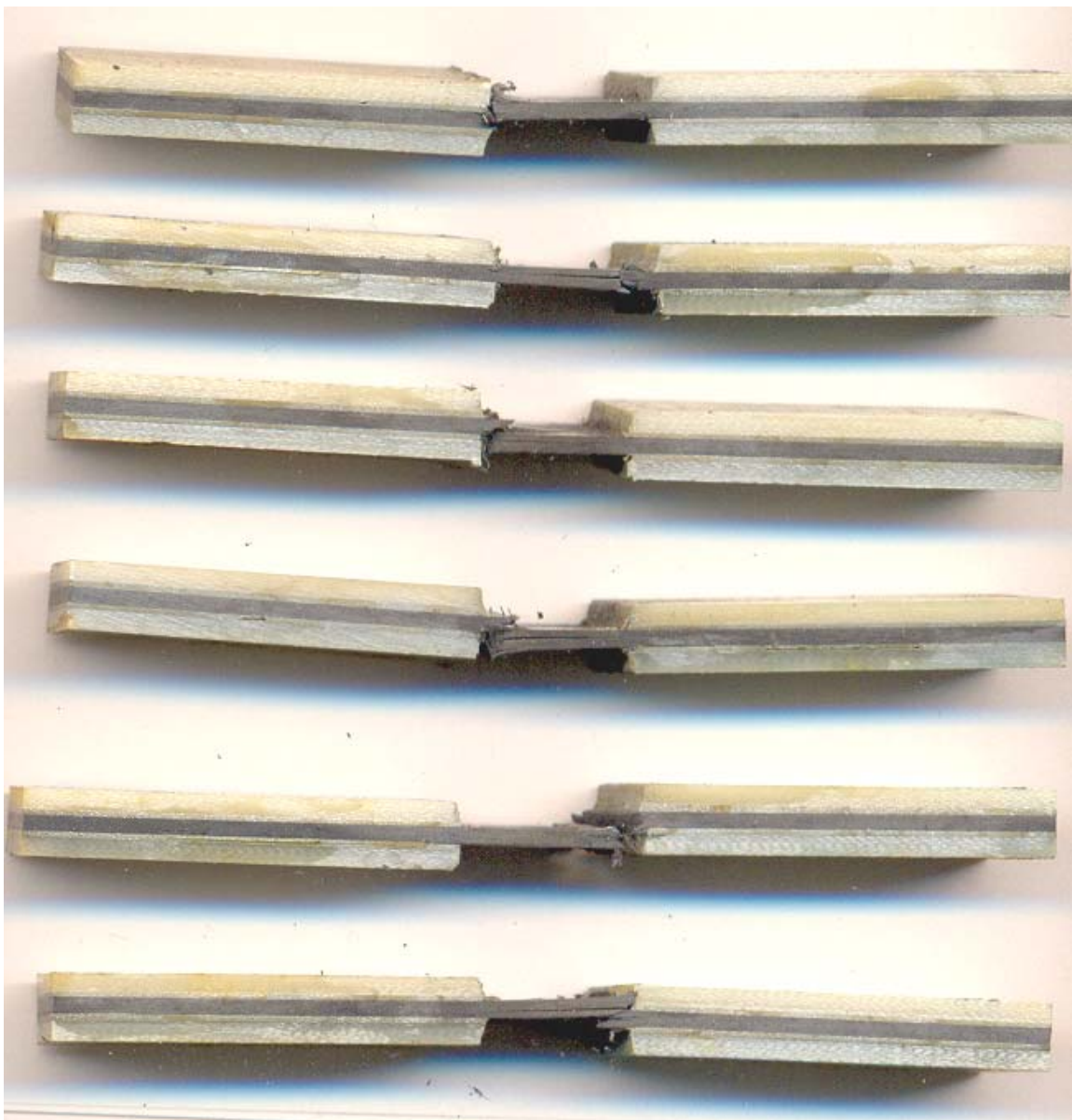
FIGURE A-3. LAMINA COMPRESSION T700G/#2510 TAPE SPECIMENS TESTED ACCORDING TO CEN prEN 2850-B/AMS SPECIFICATIONS (12.5-mm GAGE LENGTH) AT 82°C/WET CONDITIONS
