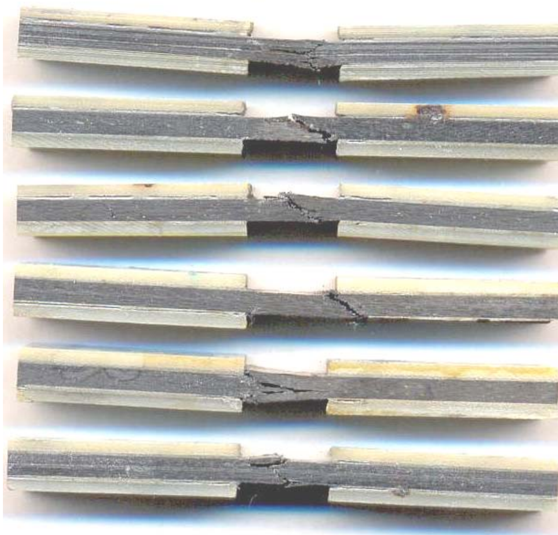
FIGURE A-7. LAMINA COMPRESSION T300/E-765 FABRIC SPECIMENS TESTED ACCORDING TO CEN prEN 2850-B/AMS SPECIFICATIONS (12.5-mm GAGE LENGTH) AT 82°C/WET CONDITIONS
