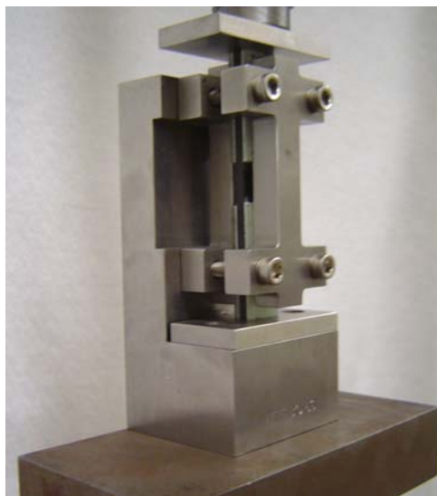
FIGURE 1. TEST FIXTURE USED FOR THE LAMINA COMPRESSION TESTS
