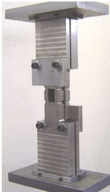
FIGURE 3. TEST FIXTURE USED FOR THE LAMINATE COMPRESSION TESTS (END LOADING)
