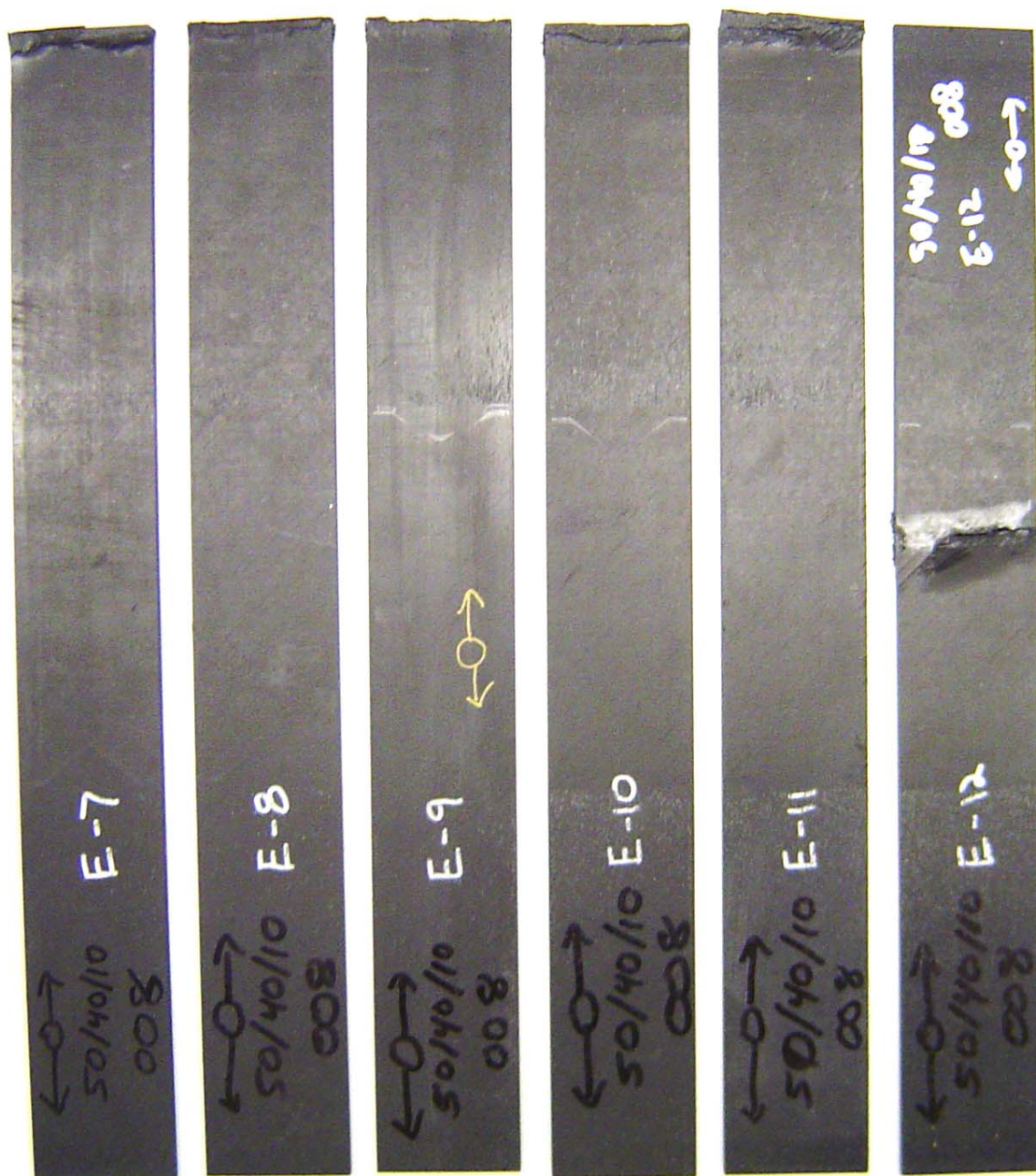
FIGURE A-13. LAMINATE COMPRESSION SPECIMENS FROM 50/40/10 TAPE LAMINATE TESTED ACCORDING TO SACMA SRM 3-94 SPECIFICATIONS (END-LOADED) AT ROOM TEMPERATURE/AMBIENT CONDITIONS
