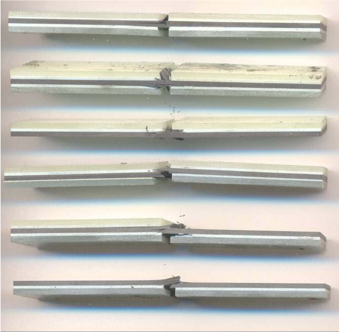
FIGURE A-2. LAMINA COMPRESSION T700G/#2510 TAPE SPECIMENS TESTED ACCORDING TO SACMA SRM 1R-94 SPECIFICATIONS (4.75-mm GAGE LENGTH) AT ROOM TEMPERATURE/AMBIENT CONDITIONS
