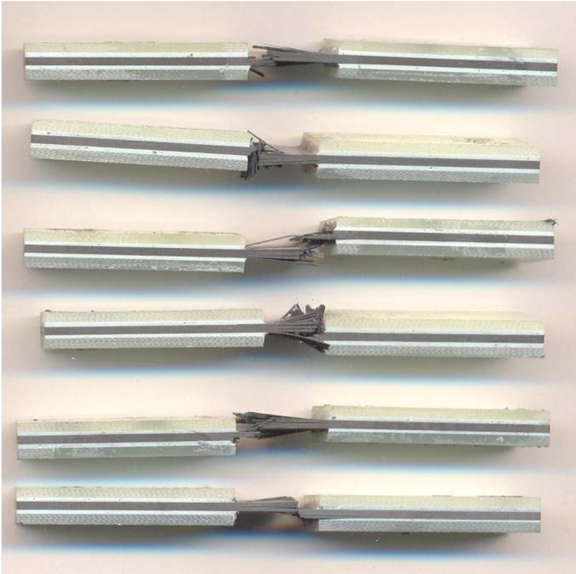
FIGURE A-1. LAMINA COMPRESSION T700G/#2510 TAPE SPECIMENS TESTED ACCORDING TO CEN prEN 2850-B/AMS SPECIFICATIONS (12.5-mm GAGE LENGTH) AT ROOM TEMPERATURE/AMBIENT CONDITIONS
