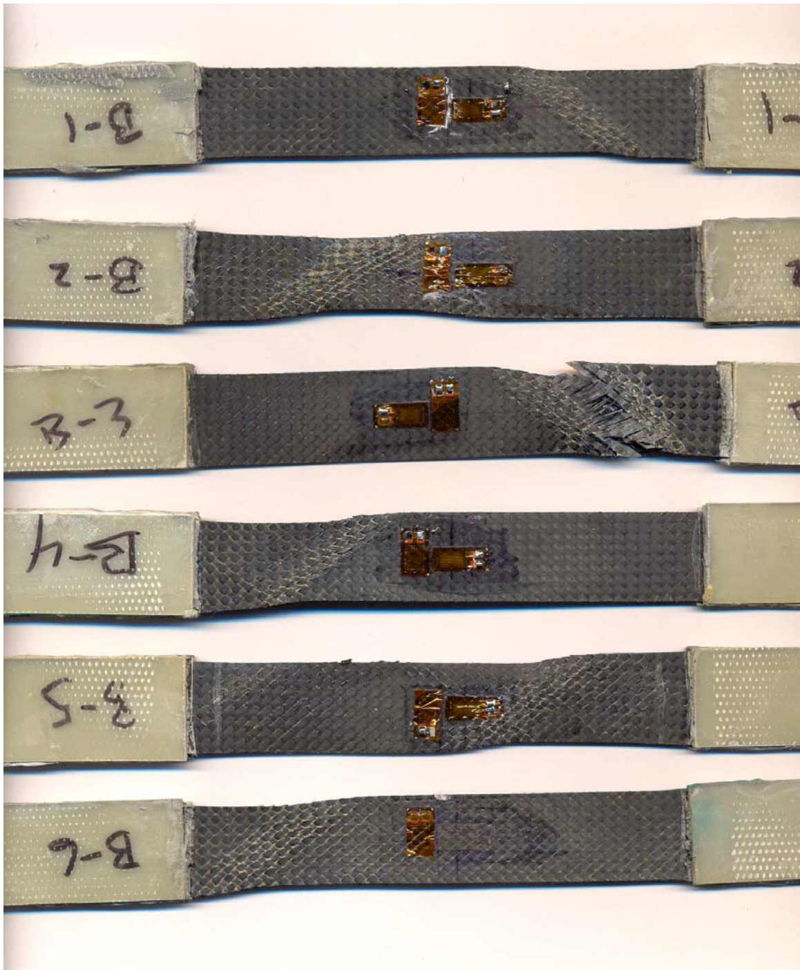
FIGURE A-34. IN-PLANE SHEAR SPECIMENS FROM EIGHT-PLY FABRIC LAMINATE TESTED AT 82°C/WET CONDITIONS
