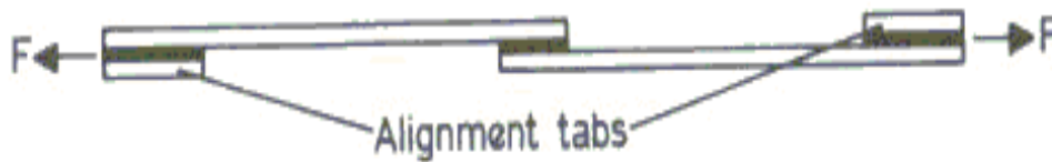
FIGURE 3-16. A SINGLE LAP JOINT WITH ALIGNMENT TABS (FROM ADAM, COMYN, AND WAKE [29])
