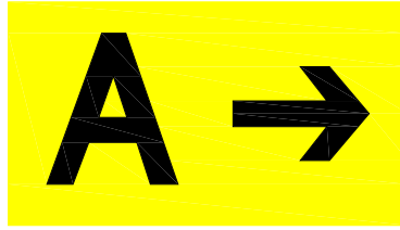
a. Direction/Runway Exit Sign
