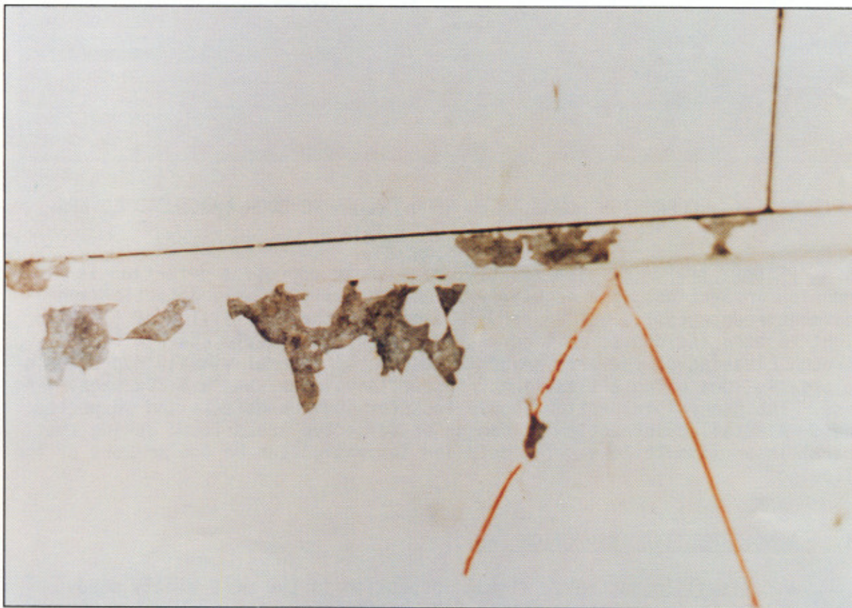
FIGURE 5-2. CORROSION UNDER CHIPPED AND LOOSE PAINT ON WING SKIN
