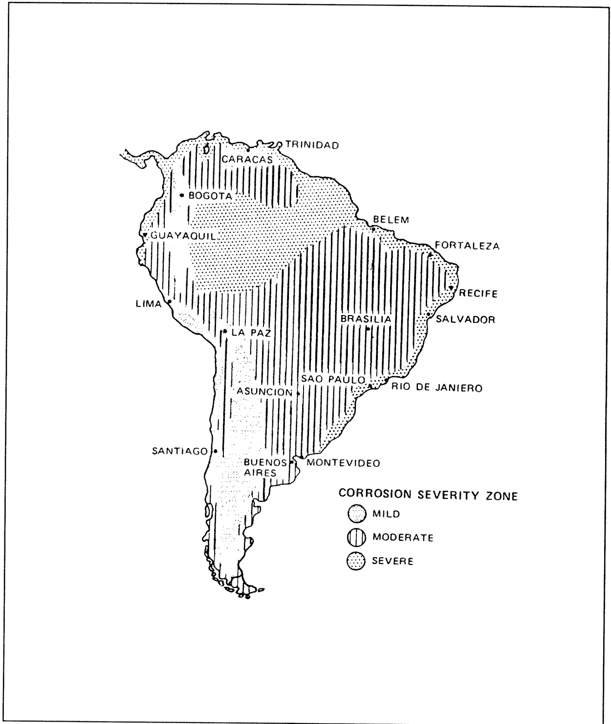
FIGURE 4-16. SOUTH AMERICA CORROSION SEVERITY MAP
