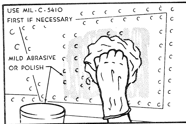
FIGURE 6-12. POLISHING AND BRIGHTENING ALCAD SURFACES
