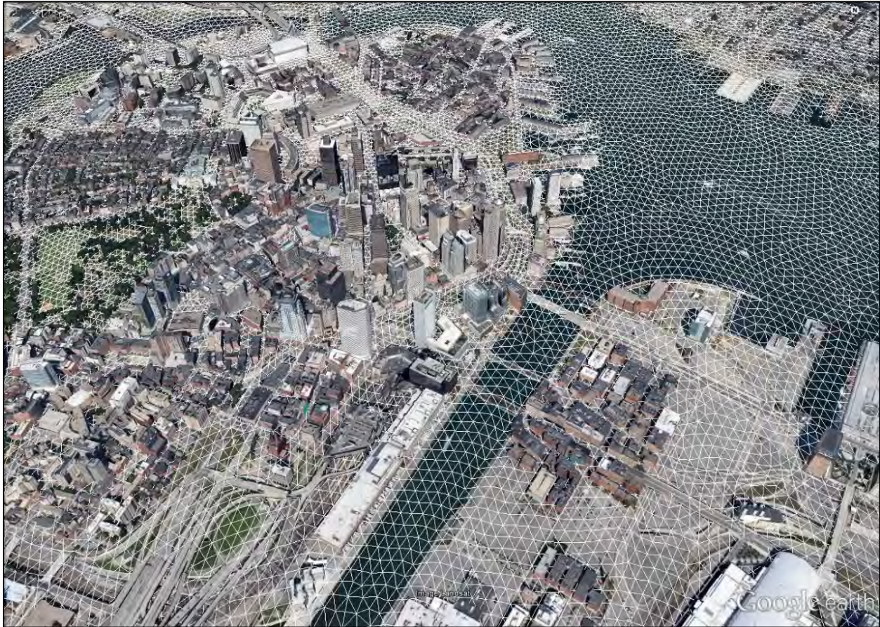
Figure 14.15. Example of the fine, highly-resolved hydrodynamic model mesh used in the Boston Central Artery/Tunnel vulnerability assessment study (from Douglas 2015; permission to use image provided by MassDOT)
