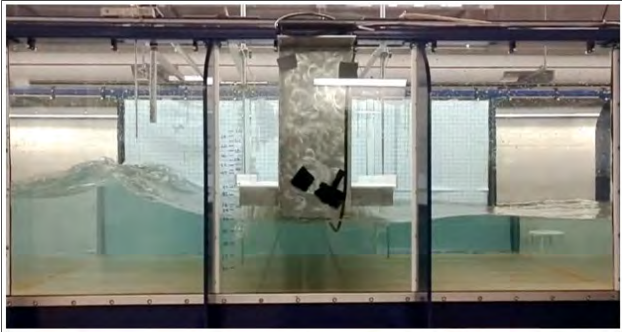
Figure 6.22. Physical model experiment on wave loads on a bridge deck in a wave flume (University of South Alabama wave flume)
