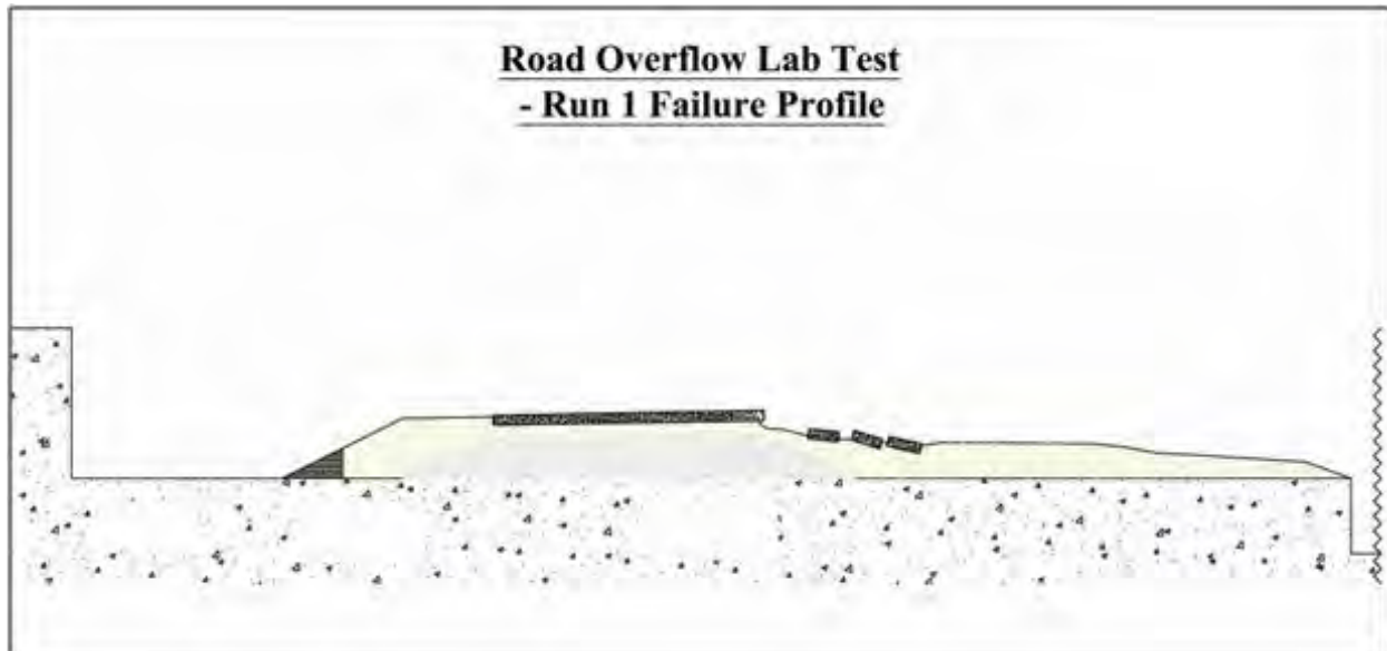
Figure 10.9. Schematic of results from USA/TAMU laboratory experiments test run one
