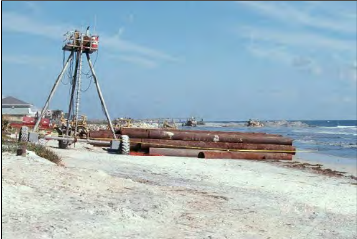
Figure 6.10. A CRAB (Coastal Research Amphibious Buggy) used to measure beach profiles during beach nourishment
