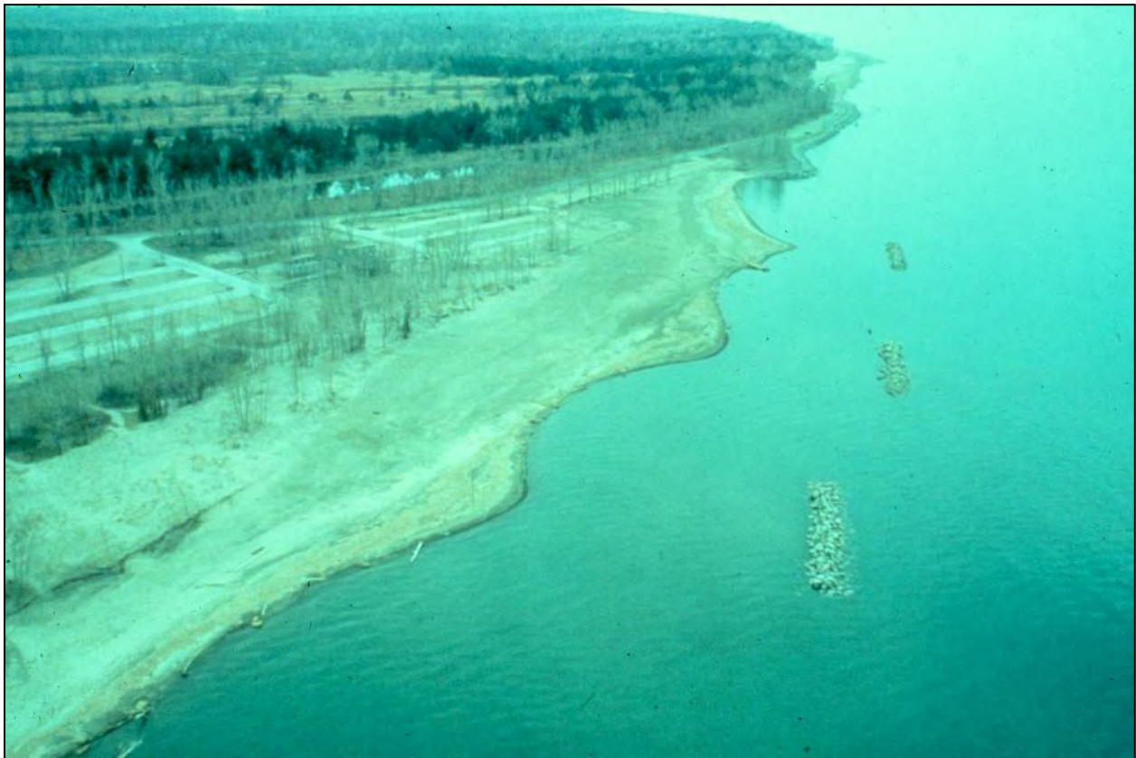
Figure 8.13. Offshore segmented breakwaters with salients in beach nourishment (Presque Isle State Park, Pennsylvania, circa 1980, USACE archive photograph)
