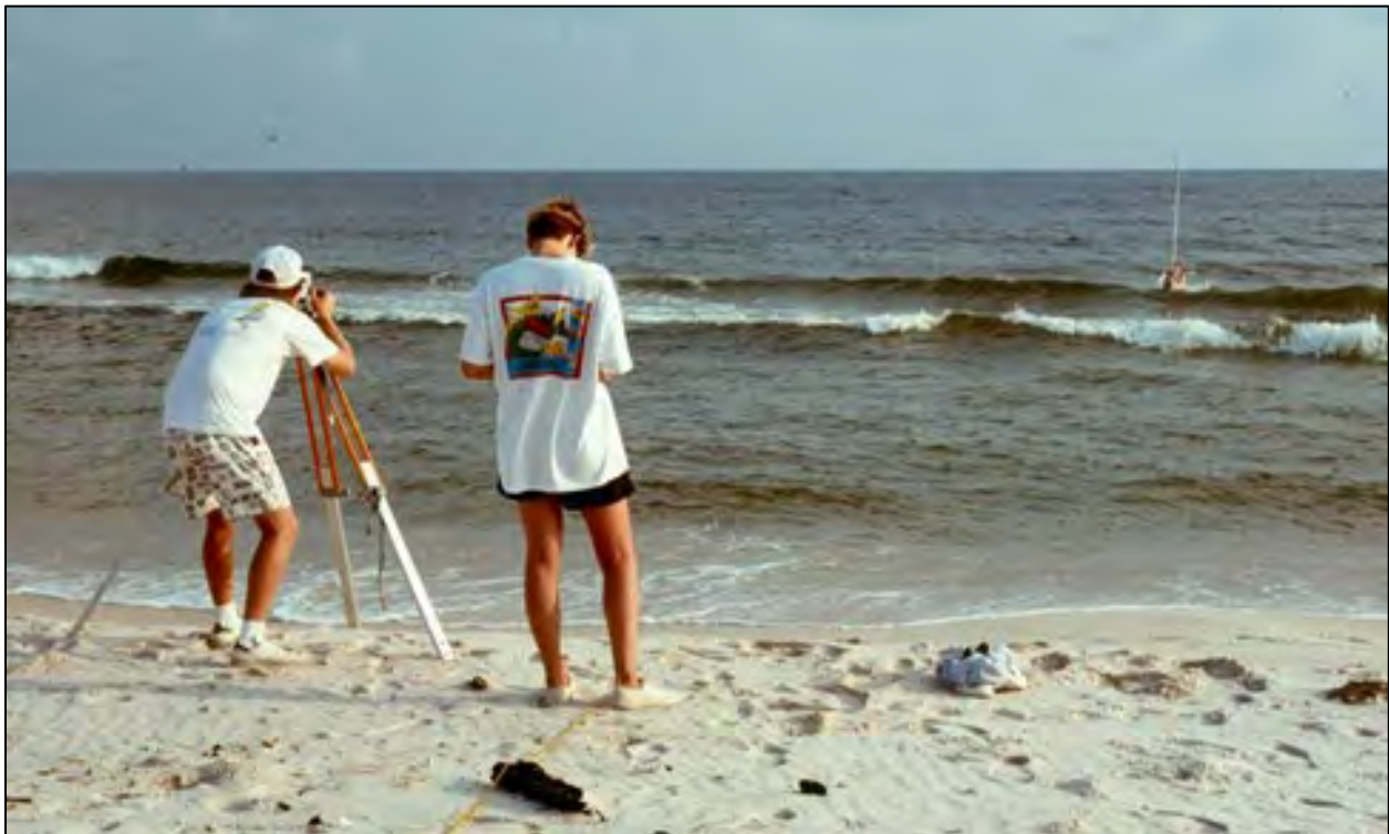
Figure 6.9. Beach profile surveying crew using a traditional level and rod
