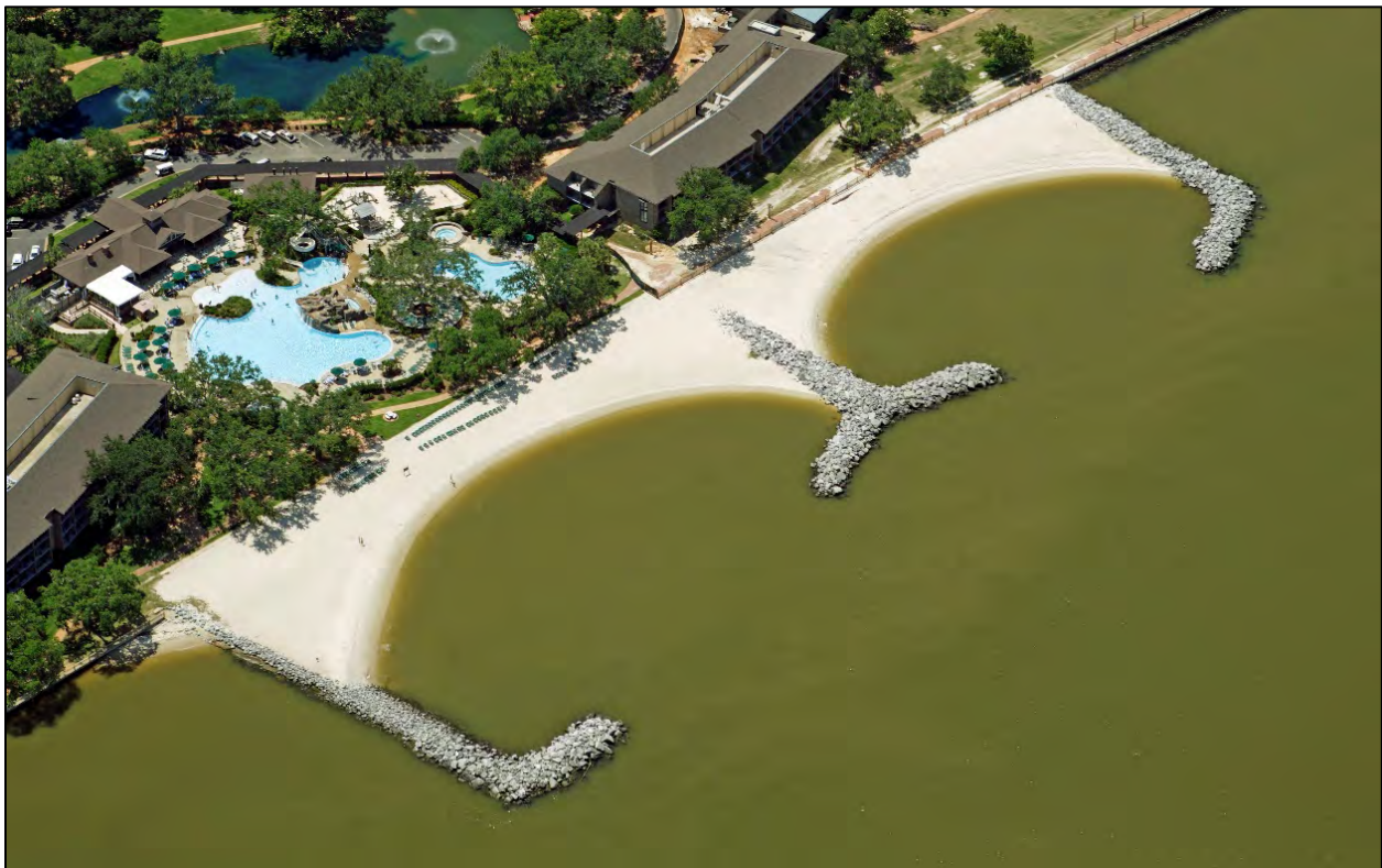
Figure 8.17. Constructed pocket beach stabilized with a T-head groin breakwater system (Point Clear, Alabama, circa 2006)
