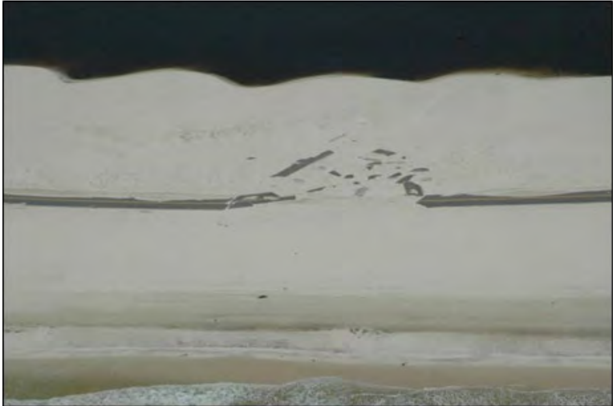
Figure 10.13. Pavement moved landward by overwash processes. (Florida SH 399, Gulf Islands National Seashore, Florida after Hurricane Ivan, 2004)
