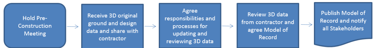
Figure 35. Flowchart. Establishing a model of record.
