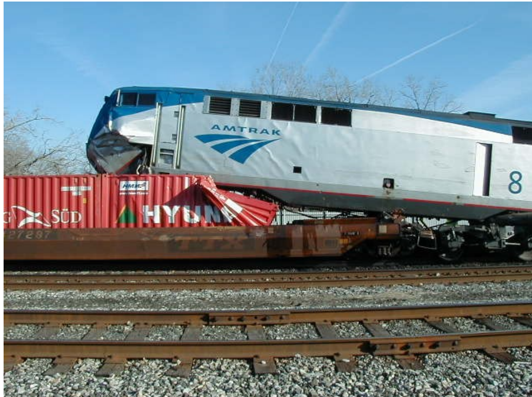
Figure 3. Amtrak locomotive resting on top of container on rear car of Norfolk Southern freight train.
