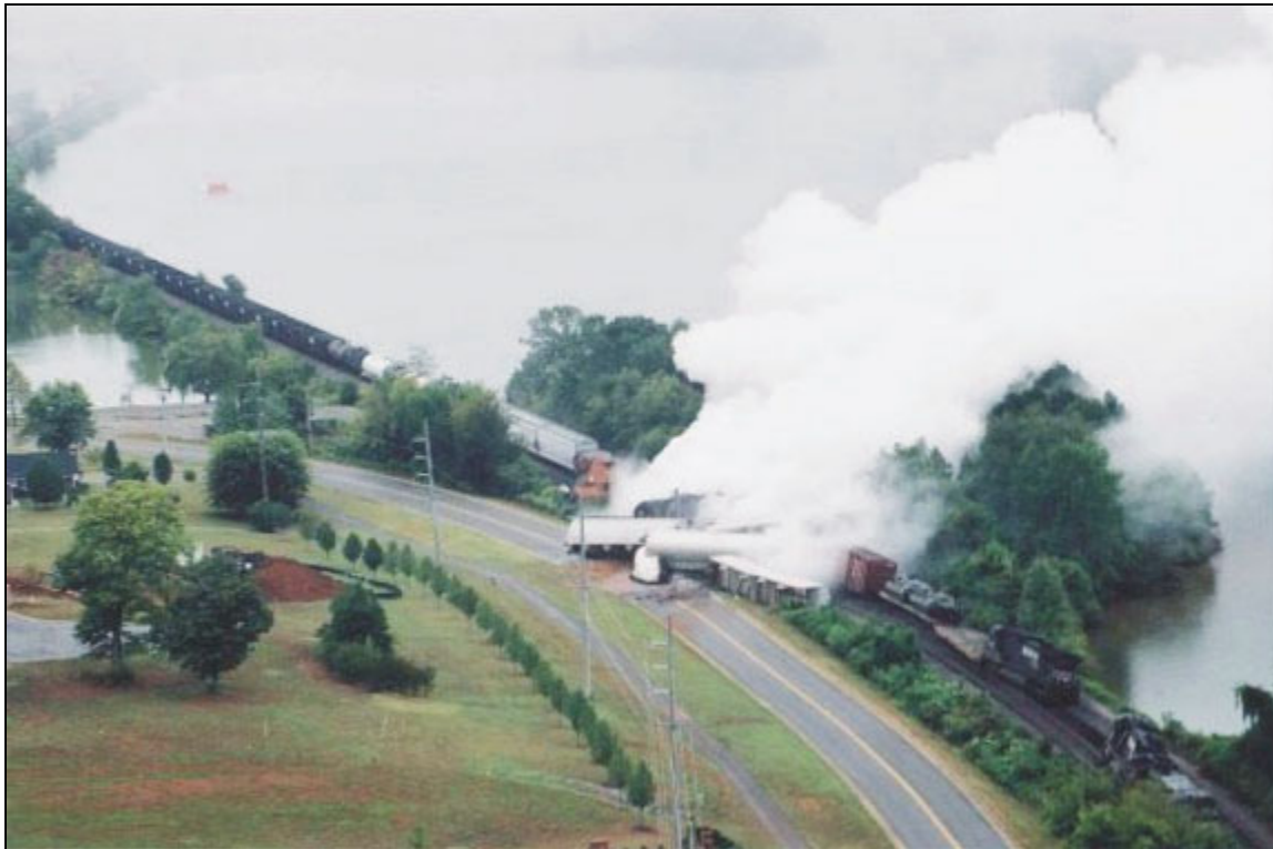
Figure 1. Looking east at the derailment of NS train 15T showing fuming sulfuric acid from ruptured tank car.
