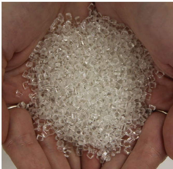
FIGURE 1. Cellulose acetate nurdles for injection molding. These colorless nurdles also contain the plasticizer diethyl phthalate. Photo by Odile Madden and Morgan Dundon, Smithsonian Institution, MCI.
