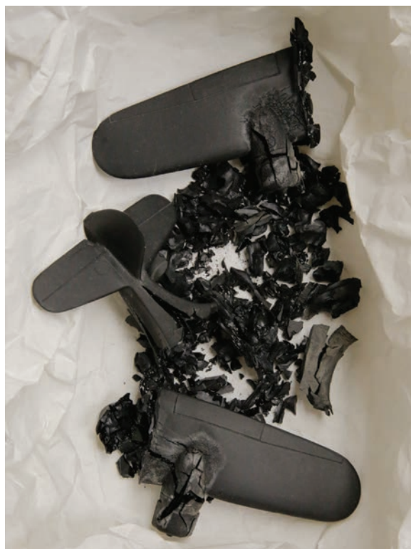
FIGURE 1. Intact (top) and deteriorated (bottom) aircraft recognition models in the National Air and Space Museum collection, Smithsonian Institution. Photos by E. Keats Webb, National Air and Space Museum, top, and Odile Madden, Museum Conservation Institute, bottom.
