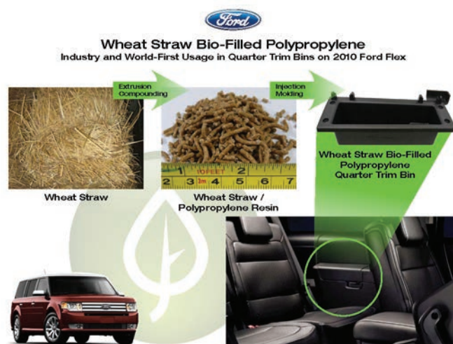
FIGURE 7. Wheat straw–reinforced polypropylene introduced in the 2010 Ford Flex third-row storage bin.
