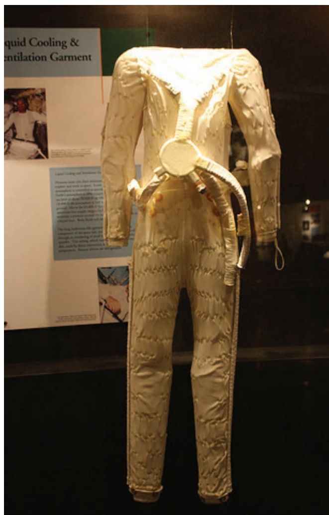
FIGURE 13. The shuttle-station LCVG. Courtesy of ILC Dover, LP.
