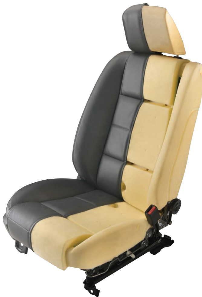
FIGURE 6. Soy-based polyurethane foam introduced in the 2008 model year Ford Mustang seat.
