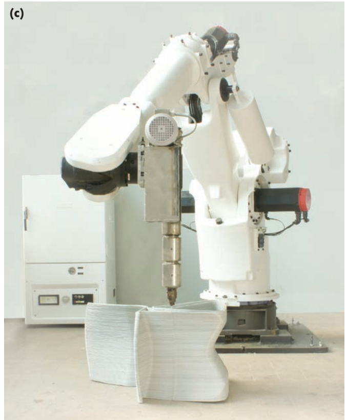
FIGURE 13. (a) Endless Chair by Dirk Vander Kooij, 2011. (b) Detail of robot printing an Endless Chair by Dirk Vander Kooij, 2011. (c) Robot printing an Endless Chair. Images courtesy of Studio Dirk Vander Kooij.
