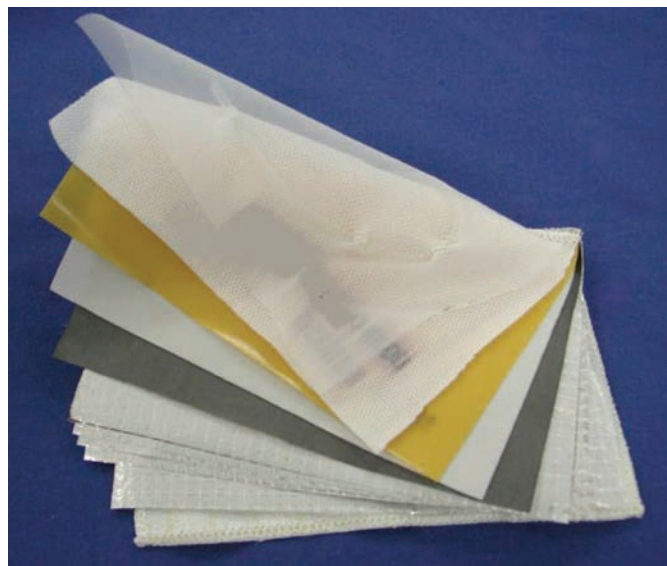
FIGURE 16. The shuttle/space station suit layers. Courtesy of ILC Dover, LP.
