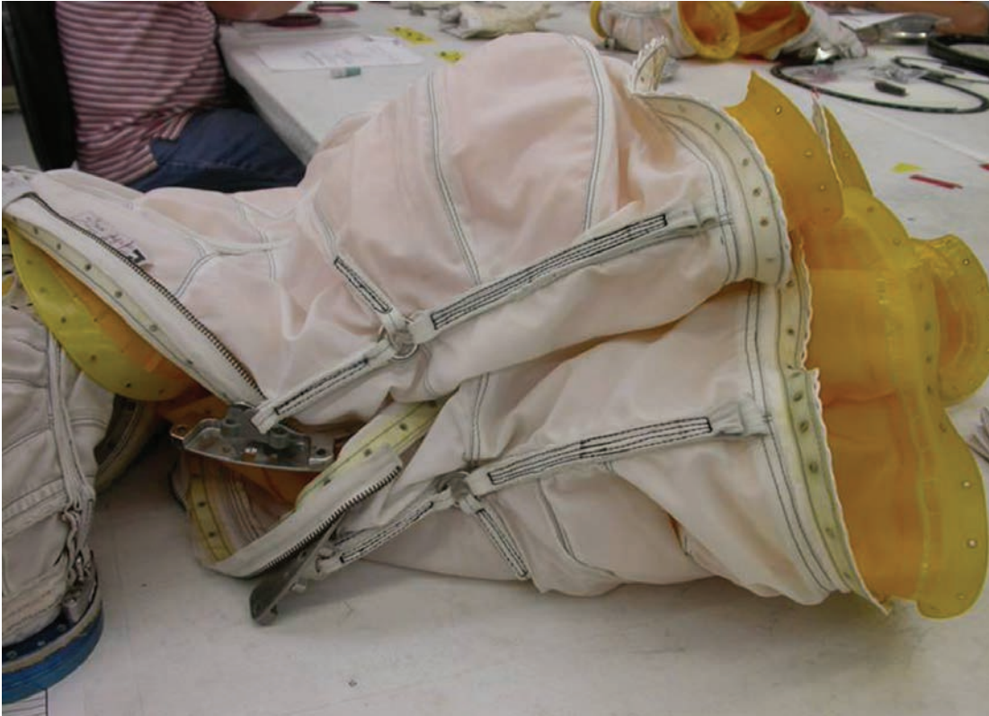
FIGURE 14. Waist subassembly including the bladder, restraint fabric, and webbings. Courtesy of ILC Dover, LP.
