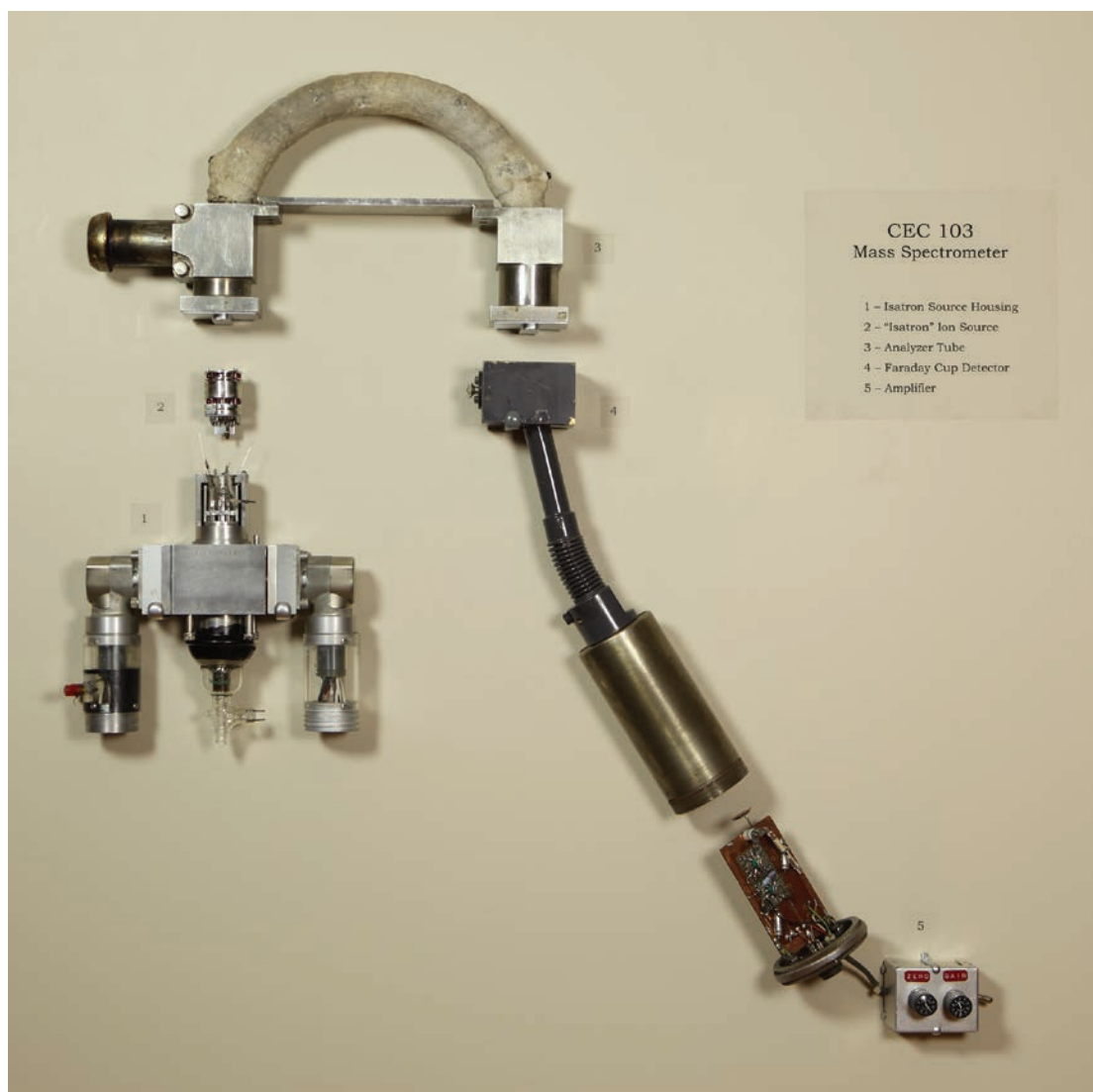
4. Image of CEC components assembled as they would have appeared in instrument. CEC 21-103, components. Gift of Charles Judson, Chemical Heritage Foundation Collections, Philadelphia PA. Photograph by Gregory Tobias.
