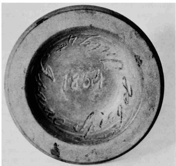
FIGURE 16.—Red earthenware mold used by Isaac Spiegel for the drape molding of small dishes; marked “Isaac Spiegel July 4th 1854.” Diameter: 9.7 cm. (Collection of the Philadelphia Museum of Art.)
