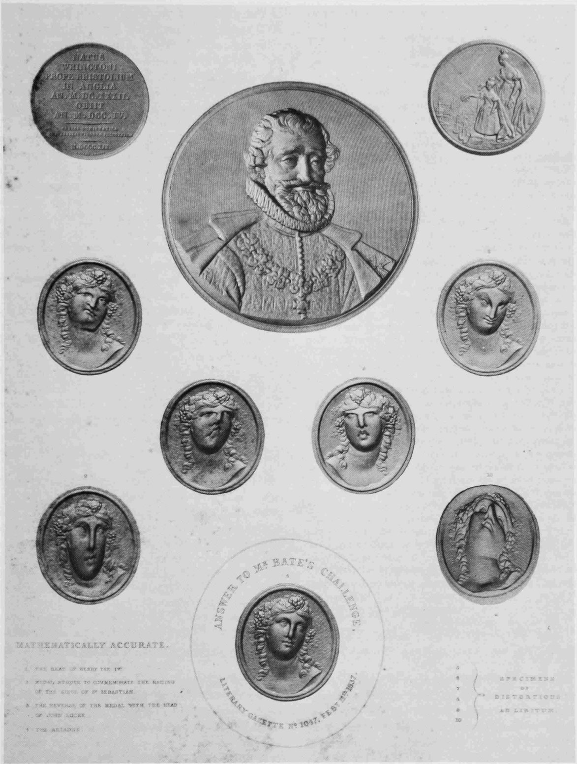
FIGURE 4.—Medal rulings executed with the Collas machine in response to a challenge from John Bate's supporters. (Courtesy Library of Congress)
